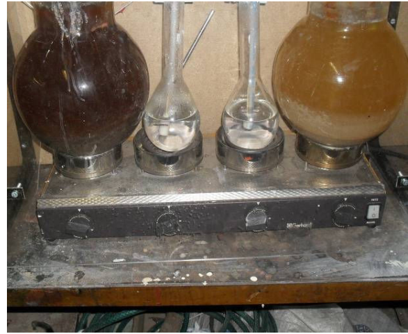
Fig. 8. Front view of the glass reservoirs filled with material suspension
