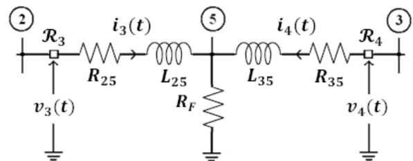
Fig. 2 Electrical scheme for a pair of synchronized relays.
