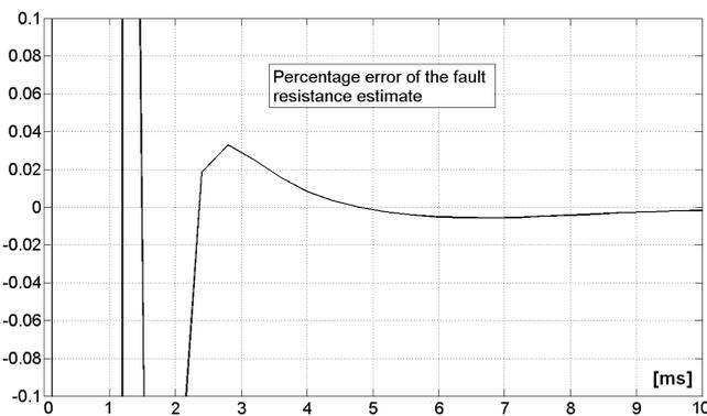
Fig. 6. Time evolution of the fault resistance percentage error.  $S_F = 900m$ ,  $R_F = 10\Omega$ .
