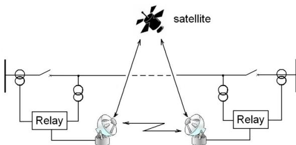
Fig. 1 Single line segment equipped with a synchronization system of GPS type.
