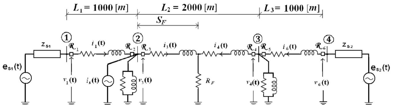
Fig. 3 The examined MV-distribution feeder with the locations of distance relays ( $\mathcal{R}_i, i = 1, \dots, 6$ ) and fault resistance ( $R_F$ );  $e_{s1}$  and  $e_{s2}$  are the main equivalent source and the equivalent of the distributed generator, respectively.
