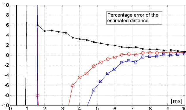
Fig. 5. Time evolution of the fault distance percentage error as computed from resistance (squares), inductance (dots), and both (circles) estimates.  $S_F = 900m$ ,  $R_F = 10\Omega$ .
