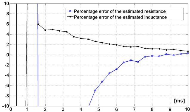
Fig. 4 Time evolution of the percentage error of  $\hat{R}_{25}$  (dots) and  $\hat{L}_{25}$  (squares).  $S_F = 900m$ ,  $R_F = 10\Omega$ .
