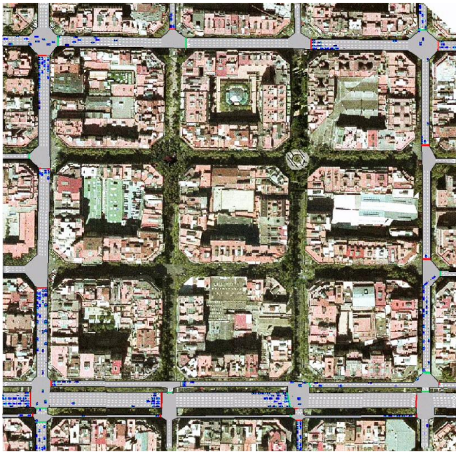
Fig.12. A superblock is comprised of 9 blocks, confined by vehicular streets; the internal connections are pedestrianized and covered by green layer. Source: Agencia de Ecología Urbana de Bar Barcelona.
