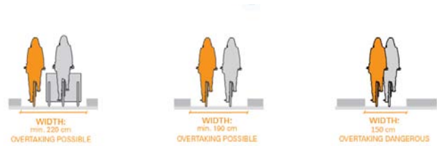
Fig.4 Bicycle lane width of the sample Picture source: Mexico_City_Gehl_toolbox
