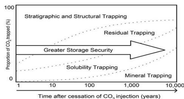
Fig.1: Trapping CO<sub>2</sub> mechanisms vs. time
