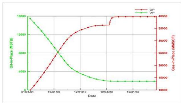
Fig. 9: homogenous reservoir storage capacity behaviour
