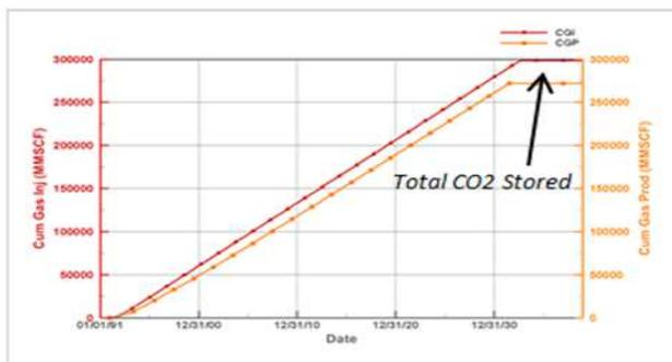
Fig. 8: Total CO<sub>2</sub> stored in fractured reservoir
