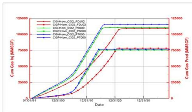
Fig. 12: Effect of the limit injection pressure in storage capacity (homogenous reservoir)
