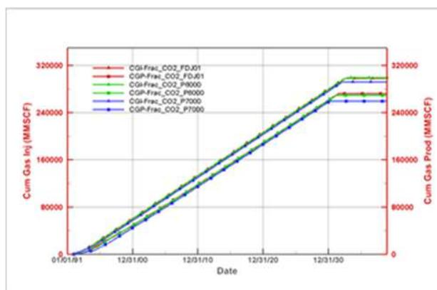
Fig. 13: Effect of the limit injection pressure in storage capacity (fractured reservoir)
