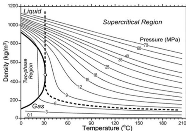
Fig. 3: Density of CO<sub>2</sub> [kg/m<sup>3</sup>] as function of temperature (obtained from Bachu, 2003)
