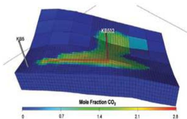
Fig. 14: Impact of the fracture conduit between Kb-5 and Kb-502 in salah project
