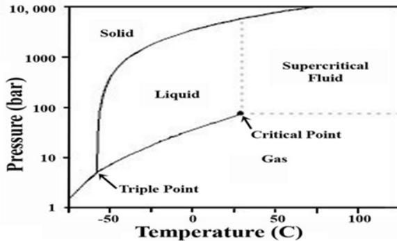
Fig. 2: CO<sub>2</sub> behaviour as a function of pressure and temperature (Critical point is at 31.1 C and 7.34 MPa), obtained from IPCC WGIII, 2005
