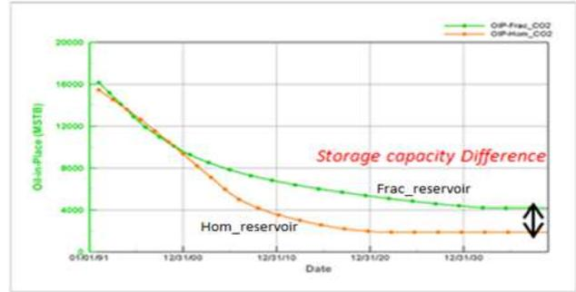
Fig. 6: Capacity storage difference between fractured and homogenous reservoir
