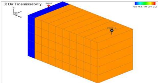
Fig. 4: 3-D simulation grid of homogenous reservoir
