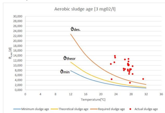
Fig. 4 Sludge ages comparison , O<sub>2</sub>= 3 mg L<sup>-1</sup>
