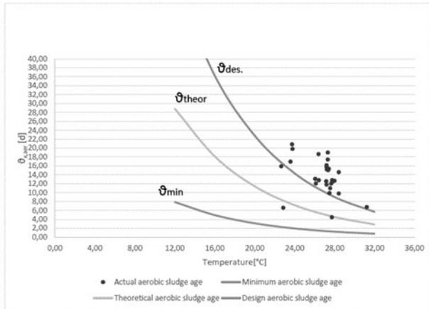
Fig 7. Process verification diagram under new plant configuration, (D.O. = 0.5 mg L<sup>-1</sup>)
