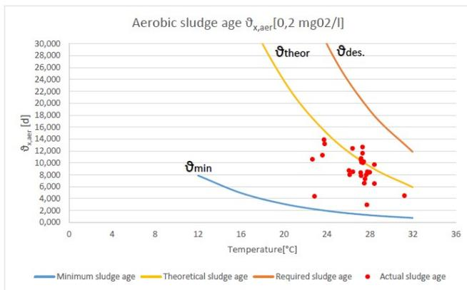
Fig. 5 Sludge ages comparison,  $O_2=0.2 \text{ mg L}^{-1}$
