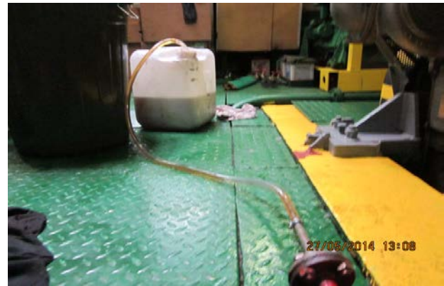
Fig. 7 Overflow from M/E to daily tank
