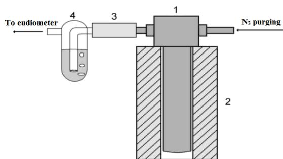
Fig.1 experimental setup for the co-pyrolysis process
