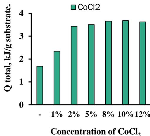
Fig. 4 the calorific value of co-pyrolysis gaseous products dependence on cobalt chloride concentration
