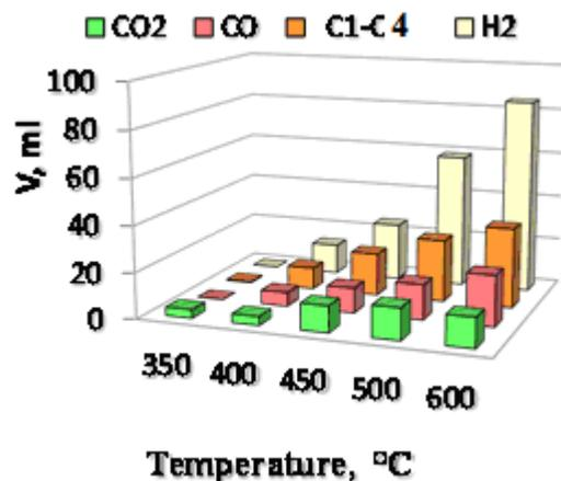
Fig. 6 The gas phase composition depending on the temperature for a non-catalytic process
