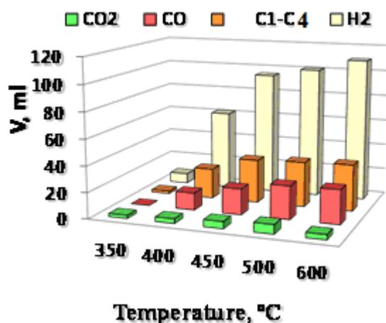
Fig. 7 the gas phase composition depending on the temperature in the presence of cobalt chloride (2% (wt.))
