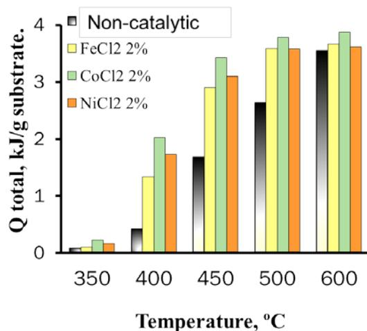
Fig. 3 the dependence of volumetric calorific value of co-pyrolysis gaseous products on the catalyst type and temperature
