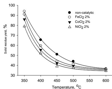
Fig. 2 the dependence of co-pyrolysis solid residue yield on the process temperature for the investigated catalysts and non-catalytic process
