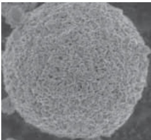
Fig. 10. Nano-Li4Ti5O12 structure [11]
