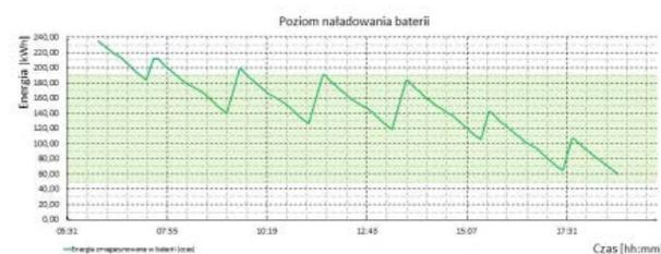
Figure 14. The charge level of an LFP battery with a capacity of 240 kWh over time
