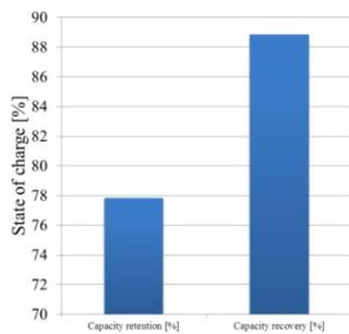
Fig. 5. Percentage of battery capacity of a KOKAM battery after 2 weeks [2]
