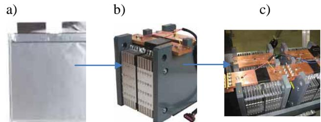
Fig. 11. Connecting a single battery (a) into one module (b), then into an energy storage system (c)
