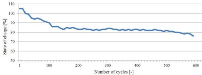
Fig. 2 The change of LFP battery capacity with the number of discharge/charge cycles [19]
