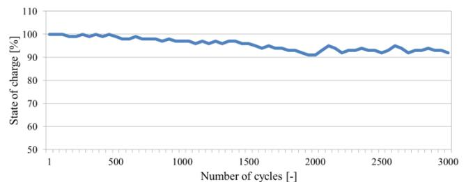
Fig. 1 The relation between the number of discharge/charge cycles and the LTO battery capacity [17]
