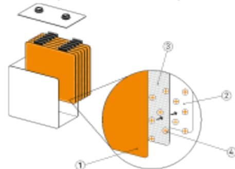
Fig. 9. Construction of a single-cell lithium-ion battery, Li-Tec: 1- cathode, 2- anode, 3- ion conductor of high molecular weight with a ceramic membrane SEPARION®, 4- lithium
