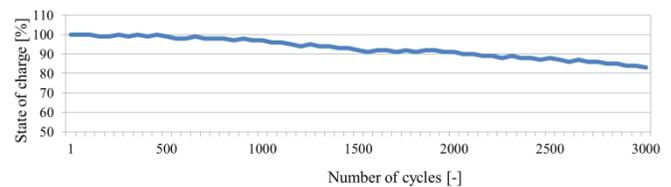
Fig. 4 The change of KOKAM battery capacity with the number of discharge/charge cycles [2]
