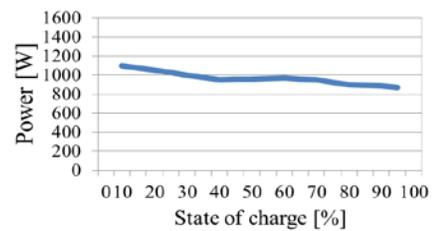
Fig. 7 The relation between battery power and the level of charge held [1]
