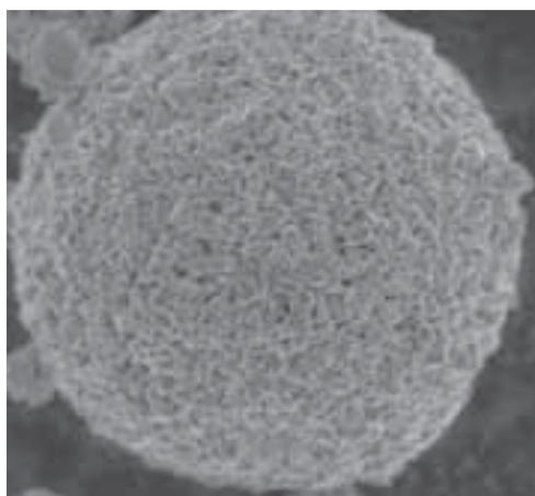
Fig. 10. Nano-Li4Ti5O12 structure [11]
