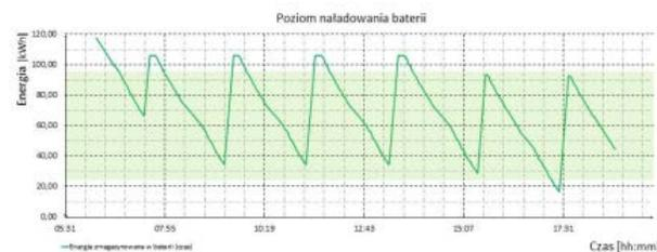
Figure 13. The charge level of an LTO battery with a capacity of 120 kWh over time
