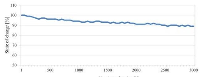
Fig. 8 The relation between the A123 battery capacity and the number of discharge/charge cycles [1]
