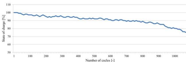
Fig. 3 The change of NMC battery capacity with the number of discharge/charge cycles [11]
