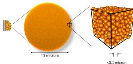
Fig. 6 Schematic visualisation of the Nanophosphate structure used in lithium-ion battery produced by A123 [2]
