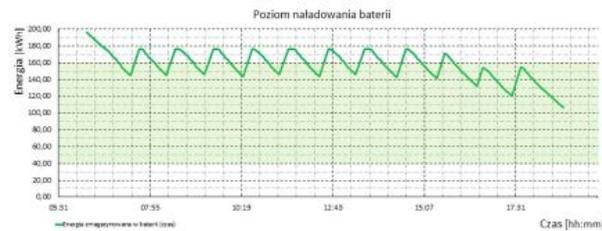
Figure 12. The charge level of an LFP battery with a capacity of 200 kWh over time
