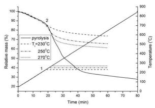
Fig.2. Rate of mass loss of wood sawdust and chicken litter pellets during heating in nitrogen at the rate of 10 °C/min.
