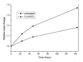
Fig.8. Relative mass change of initial and torrefied (at temperature 270 °C) pellets as a result of water vapor uptake.
