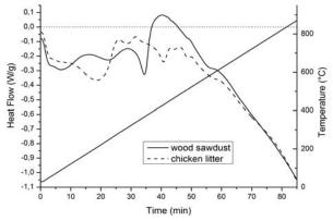
Fig.3. DSC curve of wood sawdust and chicken litter pellets in nitrogen at the heating rate of 10 °C/min.
