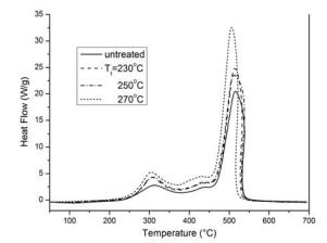
Fig.5. DSC curve of untreated and torrefied chicken litter pellets in air at the heating rate of 10 °C/min.
