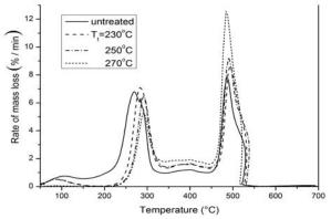
Fig.4. Rate of mass loss of untreated and torrefied chicken litter pellets during heating in air at the rate of 10 °C/min.
