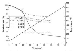
Fig.1. Change of temperature (1) and relative mass (2) of chicken litter pellets during pyrolysis and torrefaction at different temperatures Tt.
