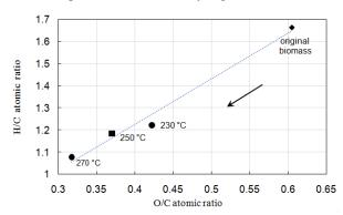
Fig.6. The atomic H/C ratio versus atomic O/C ratio in pellets, torrefied at different temperatures.
