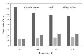
Fig.7. Changes in volatile matter, fixed carbon and ash content of pellets undergoing torrefaction at T = 230, 250 and 270 °C compared to untreated ones.
