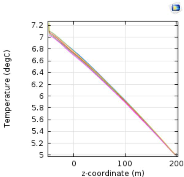
Fig. 8 Thermal response at the inlet of extraction boreholes
