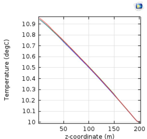
Fig. 6 Thermal response at the inlet of injection boreholes
