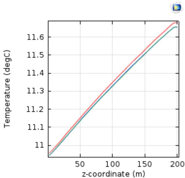
Fig. 7 Thermal response at the outlet of injection boreholes
