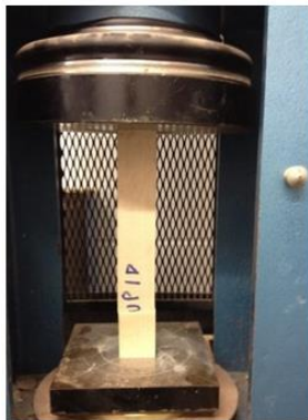
Fig. 7. Compression strength test (Source: Author)
