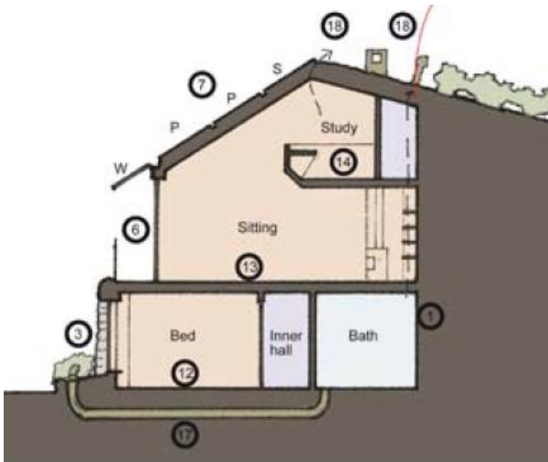
Fig. 5. Cross Section with the Earth Tube
