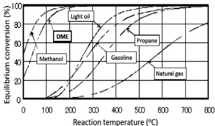
Fig. 1. Temperature dependence of equilibrium conversion of various fuels for hydrogen production by their reforming reaction [40]
