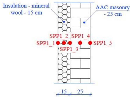
Fig. 4 Detail for exterior wall
