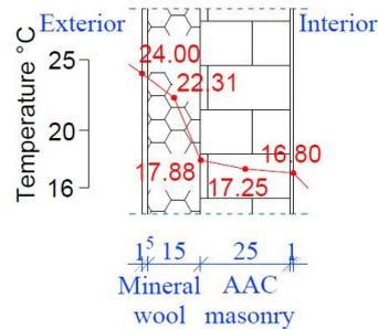
Fig. 14b Temperature distribution in the exterior wall – for the maximum exterior temperature in May 2016
