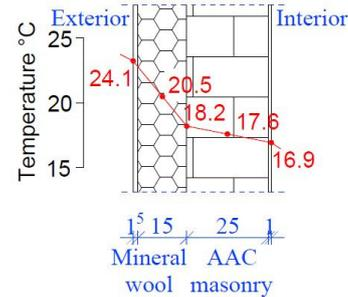
Fig. 14a Temperature distribution in the exterior wall – for the maximum exterior temperature in May 2016
