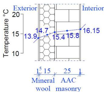
Fig. 13c Temperature distribution in the exterior wall – for the minimum exterior temperature in May 2016
