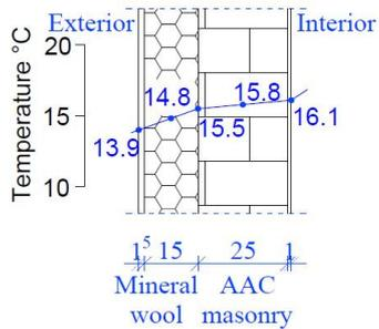
Fig. 13a Temperature distribution in the exterior wall – for the minimum exterior temperature in May 2016
