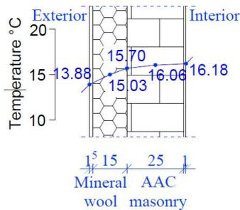
Fig. 13b Temperature distribution in the exterior wall – for the minimum exterior temperature in May 2016
