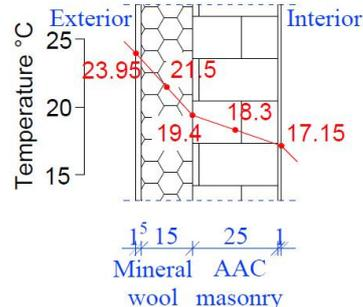
Fig. 14c Temperature distribution in the exterior wall – for the maximum exterior temperature in May 2016
