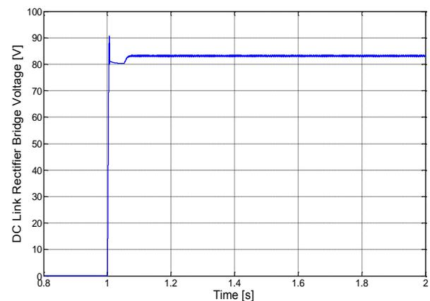
Fig. 6 The *dc* link rectifier bridge voltage
