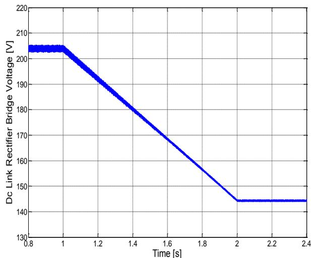
Fig. 9 The dc link rectifier bridge voltage
