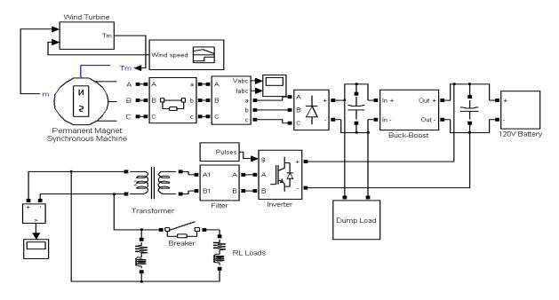
Fig. 2 Simulink diagram of the wind system.
