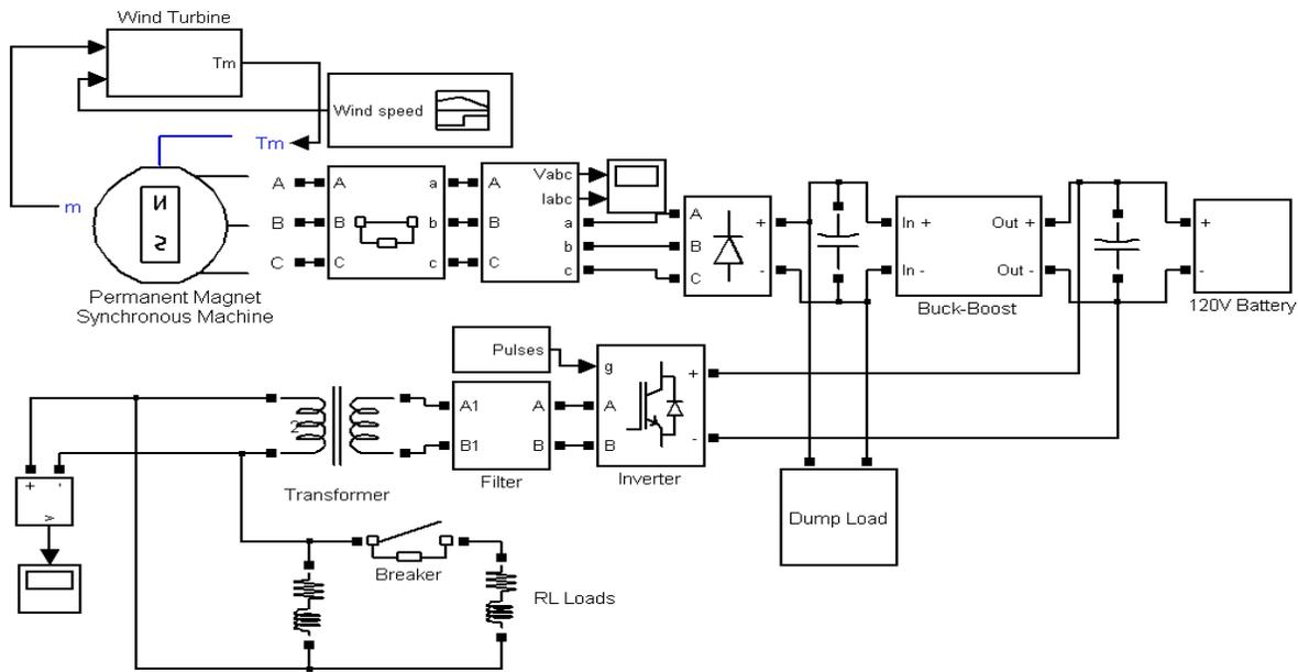
Fig. 2 Simulink diagram of the wind system.
