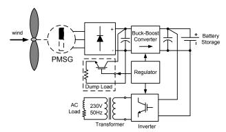
Fig.1 Wind turbine system configuration.
