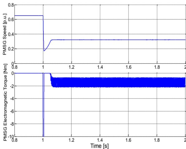
Fig. 4 PMSG rotor speed and electromagnetic torque
