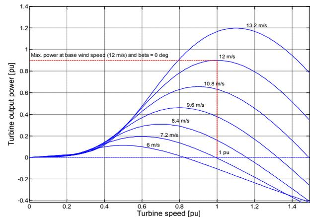
Fig. 3 Wind turbine characteristics at 3 kW
