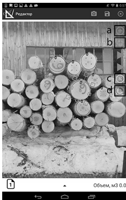
Fig. 5 manual edit; tools: a) add object b) delete object c) top label d) butt label
