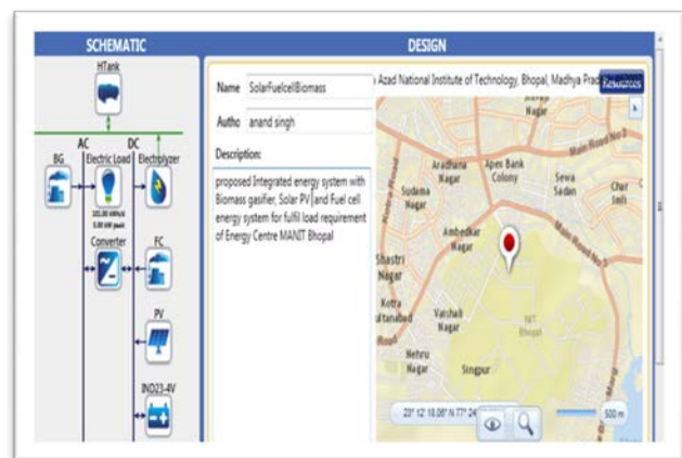
Figure.4. HOMER Simulation model of Solar PV, Biomass gasifier generator set, and Fuel cell Hybrid Energy System
