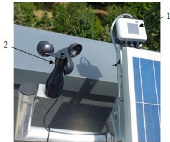
Fig. 9. Equipment for measuring weather parameters: 1- pyranometer; 2- anemometer.
