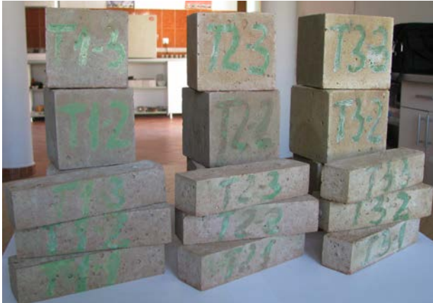
Figure 3. Pieces of burned lightweight concrete.
