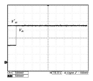
Fig.9. Experimental APF results with Feedback linearized DC voltage  $V_{dc}$  (V) and DC reference voltage  $V_{dc}^*$  (V),Ch3 and Ch4 scale: 100 V/div. Evaluation of the gain  $G_I$  of AFC, Ch2 5A/div. Time scale:10s/div.
