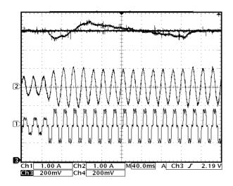
Fig. 8. Experimental APF results with PI: load current  $i_L$  (A), source current  $i_S$  (A), DC voltage  $V_{dc}$  (V) and DC reference voltage  $V^*_{dc}$  (V). Ch1 and Ch2 scale: 5 A/div; Ch3 and Ch4 scale: 40 V/div. Time scale: 40 ms/div.
