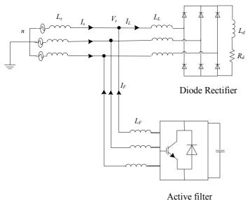
Fig 1. Power System Configuration.
