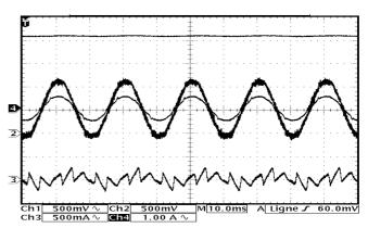
Fig. 6. Experimental results with AFC: filter current  $i_F$  (A), source current  $i_S$  (A) , source voltage Vs (V) and DC voltage  $V_{dc}$  (V). Ch3 and Ch4 scale: 5 A/div; Ch2 scale: 100 V/div; Ch1 scale: 80 V/div; Time scale: 10 ms/div.
