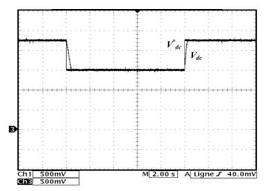
Fig.12. Experimental APF results with Feedback linearized: DC voltage  $V_{dc}$  (V) and DC reference voltage  $V^*_{dc}$  (V),Ch3 and Ch4 scale: 100 V/div,Time scale: 2s/div.
