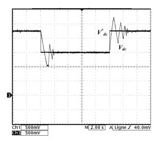
Fig.12. Experimental APF results with PI: DC voltage  $V_{dc}$  (V) and DC reference voltage  $V^*_{dc}$  (V),Ch1 and Ch3 scale: 100 V/div, Time scale: 2s/div.
