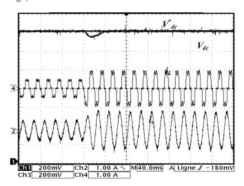
Fig. 7. Experimental APF results with Feedback linearized: load current  $i_L$  (A), source current  $i_S$  (A), DC voltage  $V_{dc}$  (V) and DC reference voltage  $V^*_{dc}$  (V).Ch1 and Ch2 scale: 5 A/div; Ch3 and Ch4 scale: 40 V/div. Time scale: 40 ms/div.
