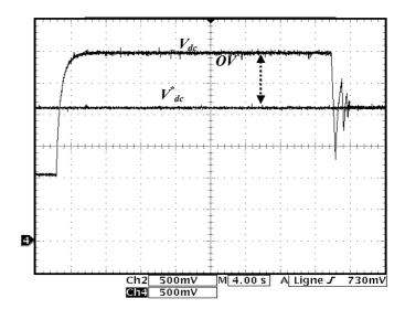
Fig. 10.Experimental APF results with PI: DC voltage  $V_{dc}$  (V) and DC reference voltage  $V^*_{dc}$  (V),Ch2 and Ch4 scale: 100 V/div. Time scale: 4 s/div.
