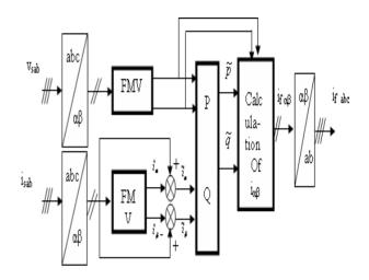
Fig. 3: The Method of Instantaneous Active and Reactive Power
