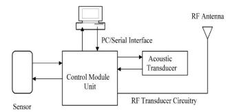
Fig. 2 Aqueous sensor setup incorporating an rf transceiver and acoustic tranducer [7].
