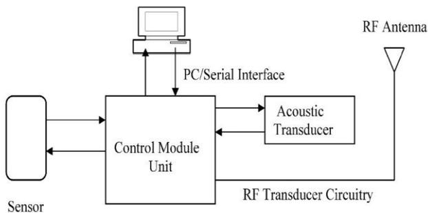
Fig. 2 Aqueous sensor setup incorporating an rf transceiver and acoustic transducer [7].
