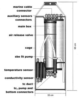
Fig. 5 CTD SBE 9 plus (adapted from Sea-Bird's Electronics Inc. catalog).
