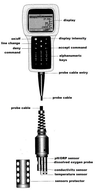
Fig. 4 YSI handheld probe model 556 (Adapted from Yellow Spring Instruments Manual).
