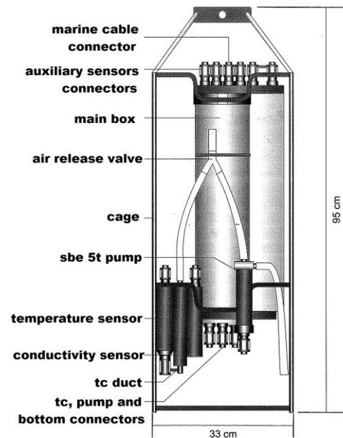
Fig. 5 CTD SBE 9 plus (adapted from Sea-Bird's Electronics Inc. catalog).
