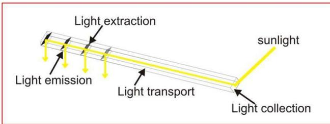
Fig 12. Horizontal Light Pipes
