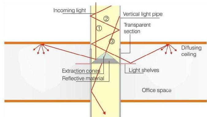
Fig 10. Light Distribution for Vertical Light Pipes
