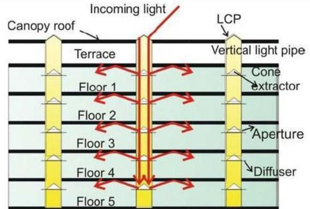
Fig 9. Vertical Light Pipes
