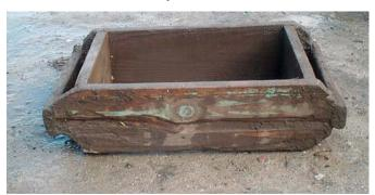
Fig. 8 Contemporary wooden mold for formatting adobe bricks.
