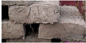
Fig. 7 Contemporary adobe bricks exposed for drying in open air in the yard of a local.
