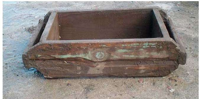
Fig. 8 Contemporary wooden mold for formatting adobe bricks. Utensil used by the same local.
