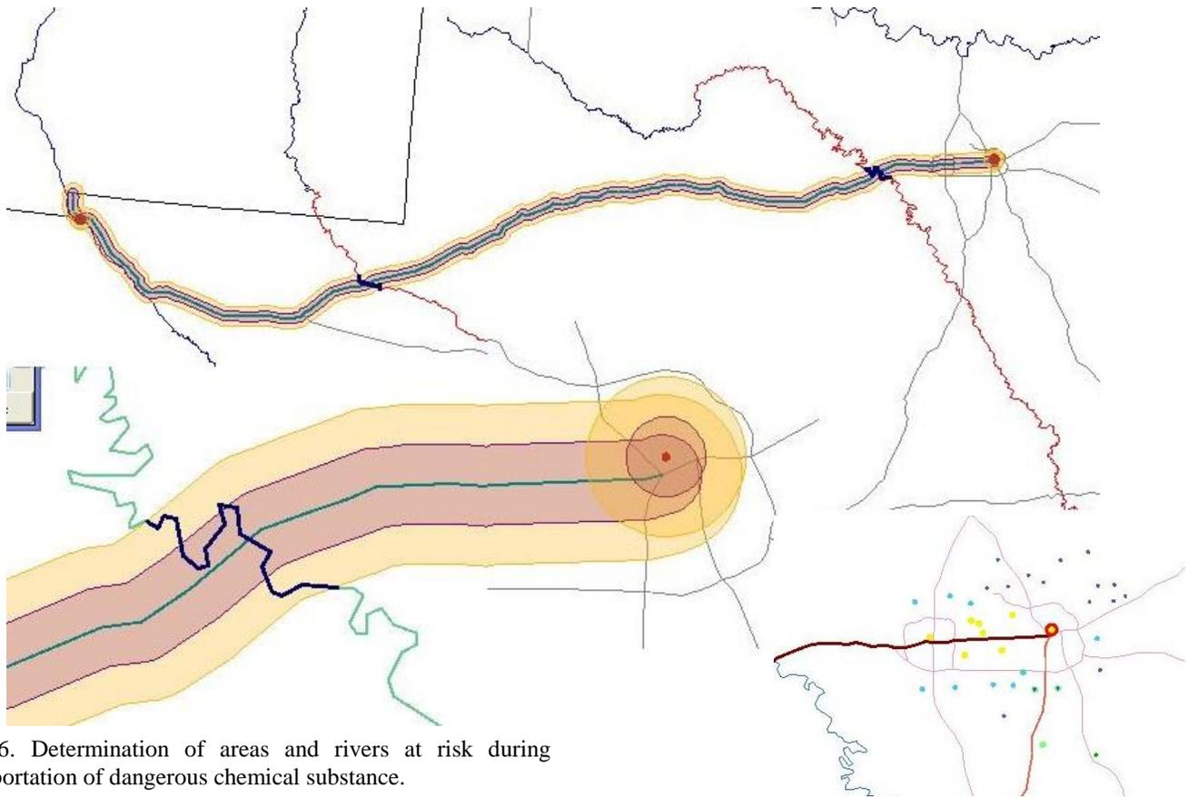
Fig. 6. Determination of areas and rivers at risk during transportation of dangerous chemical substance.
