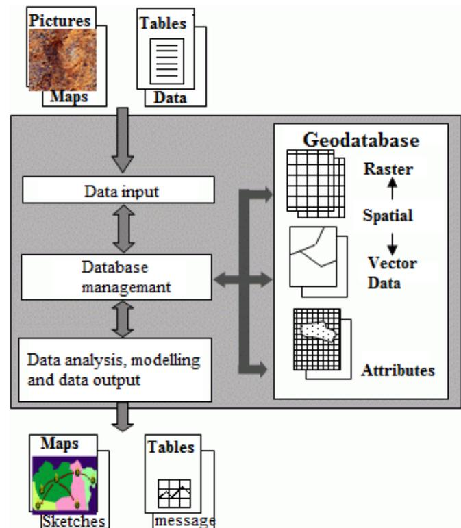
Fig.2. The basic scheme of the GIS [8]
