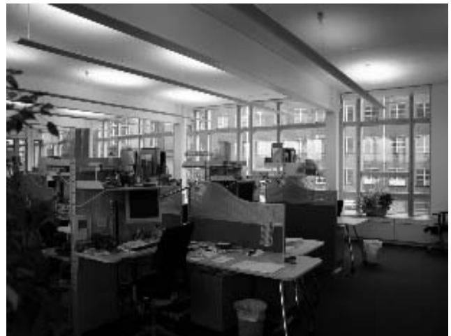
Fig.11 North façade open plan office space while south façade blinds are closed and electrical lighting is switched on during a sunny summer day
