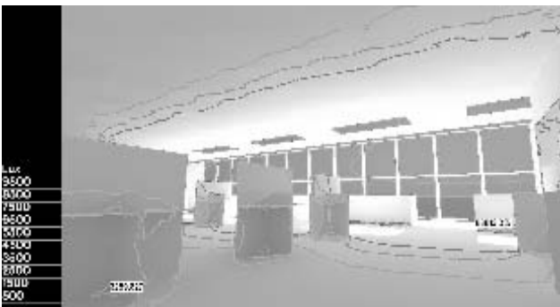
Fig.17 Daylight illuminance distributions (lux) across an open plan office floor in July with sunny sky (southeast view).
