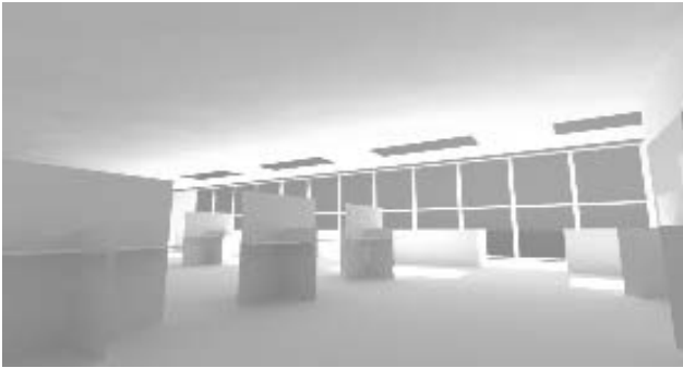
Fig.16 Lighting simulation across an open plan office floor in July under sunny sky conditions, window blinds closed (southeast view)
