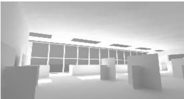
Fig.18 Lighting simulation across an open plan office floor in July under sunny sky conditions, window blinds closed (southwest view).
