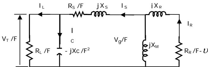
Fig.1 Per-phase equivalent circuit of SEIG
