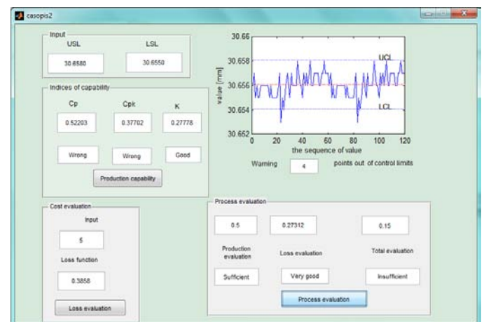
Fig. 17 Evaluation of observed production process
