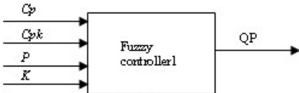
Fig.3 Block diagram of the production process control using a Fuzzy controller1
