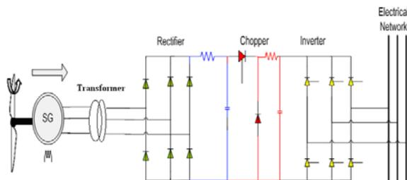
Fig.1. Wind electrical conversion system based on synchronous machine
