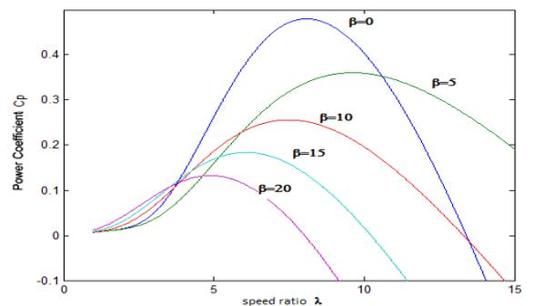
Fig.3. Power coefficient  $C_p$  as a function of  $\beta$  and  $\lambda$
