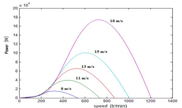
Fig.4. The characteristics of the mechanical power as function of the turbine speed.
