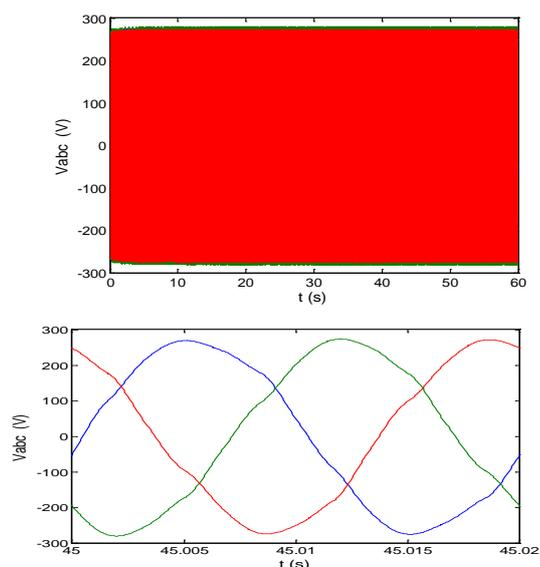
Fig. 12. The voltage in the grid phase with controller,
