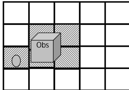
Fig. 1 an example of a square cellule grid navigation
