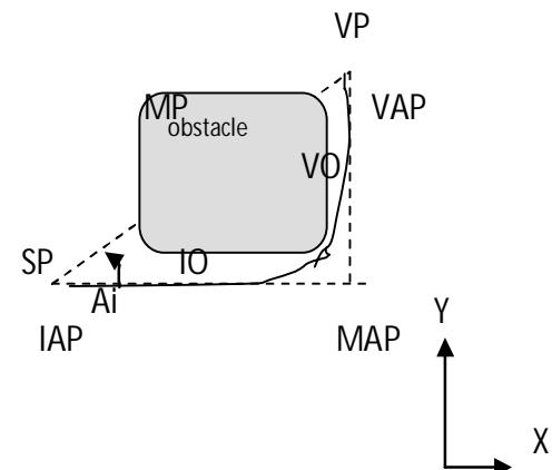
Fig. 3 Robot obstacle mode avoidance
