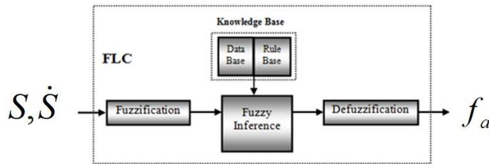
Fig. 4 Fuzzy logic control architecture
