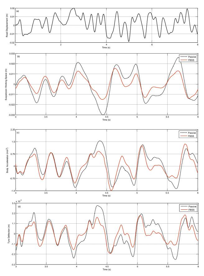
Fig. 9 The passive and active vehicle suspension systems performance under uncertain parameters. a- Road Displacement b- SWS c- BA d- DTL
