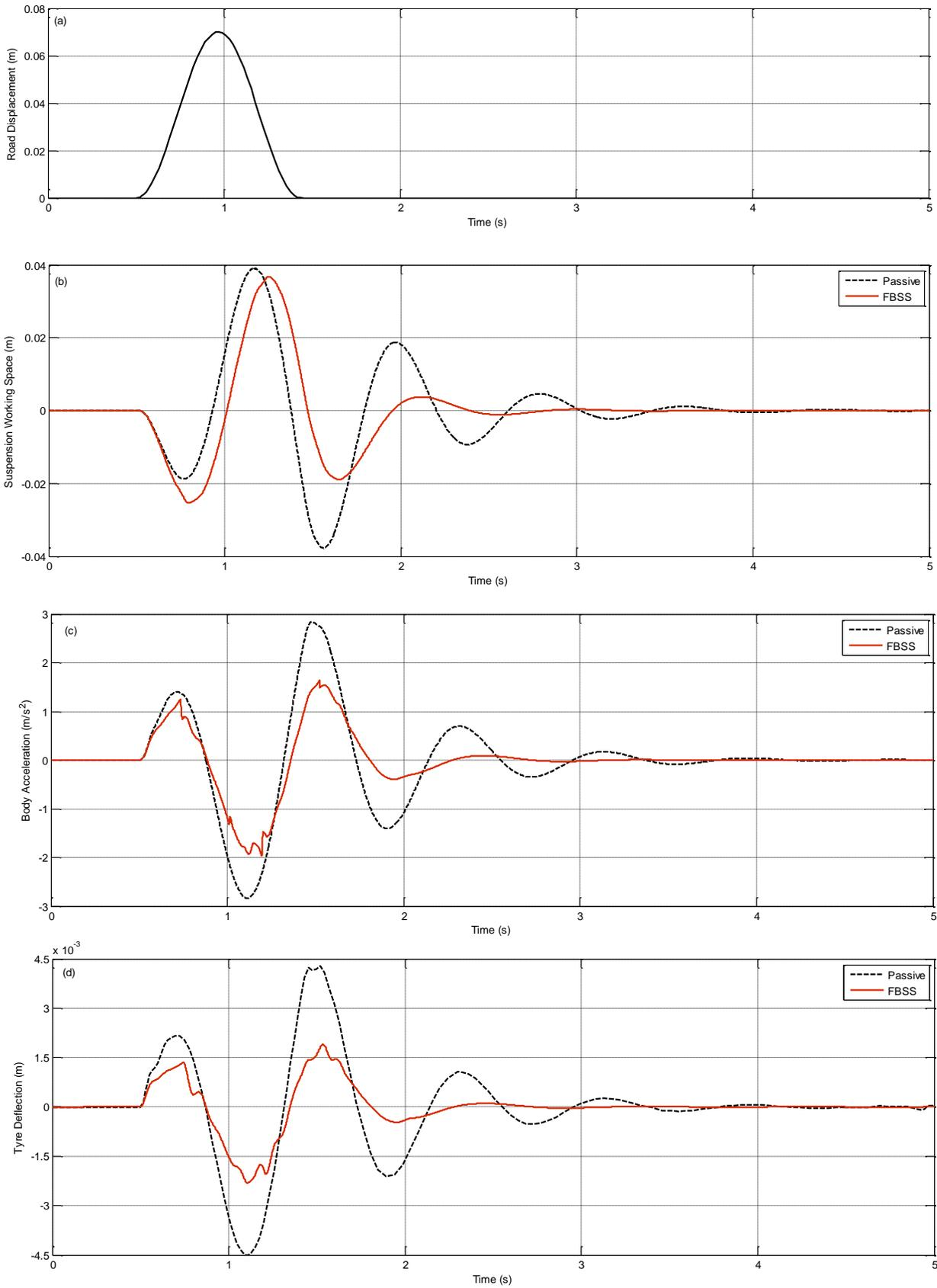
Fig. 7 The passive and active vehicle suspension systems performance under road bump excitation.
