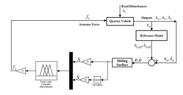
Fig. 2 The proposed FBSS controller for active vehicle suspension
