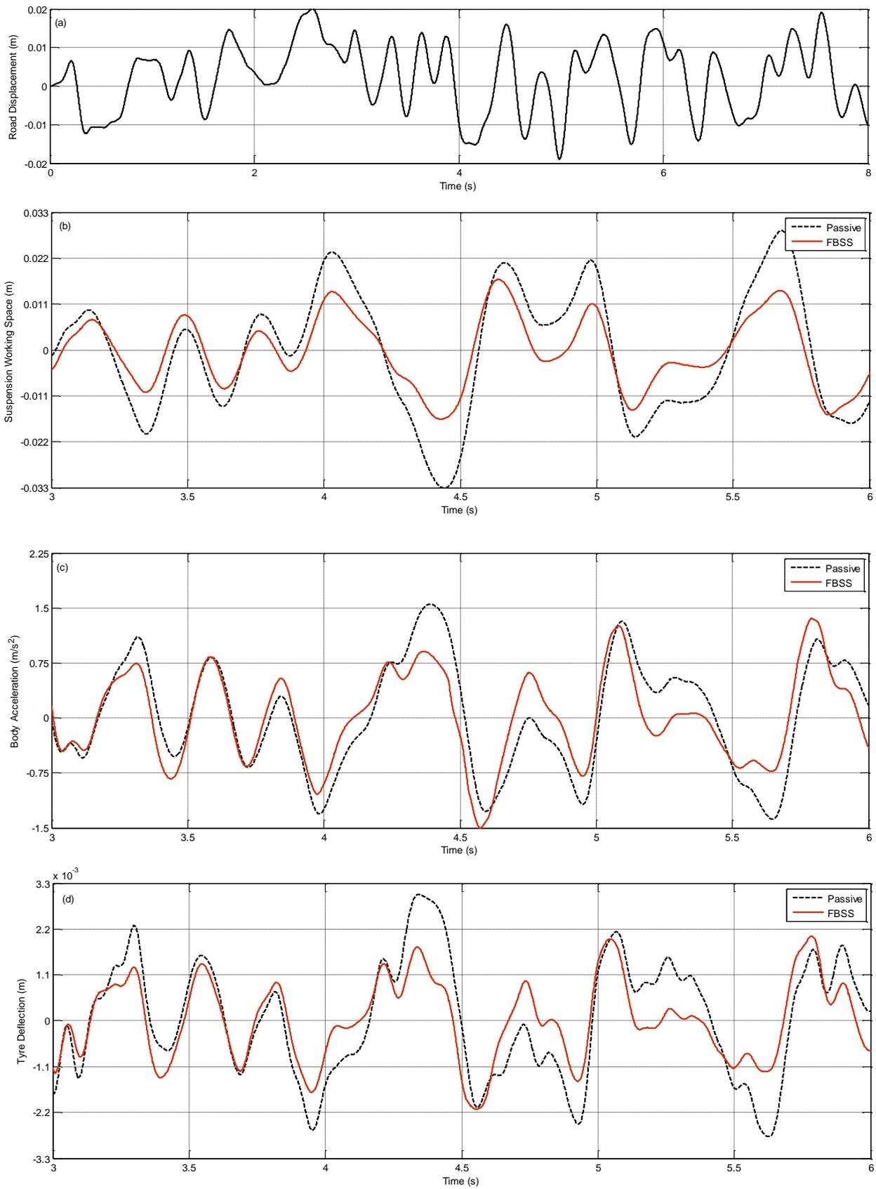
Fig. 9 The passive and active vehicle suspension systems performance under uncertain parameters.
