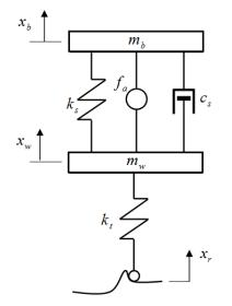
Fig. 1 Quarter vehicle active suspension model.
