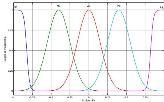
Fig. 5 Membership function of  $S$ ,  $\dot{S}$  and  $f_a$
