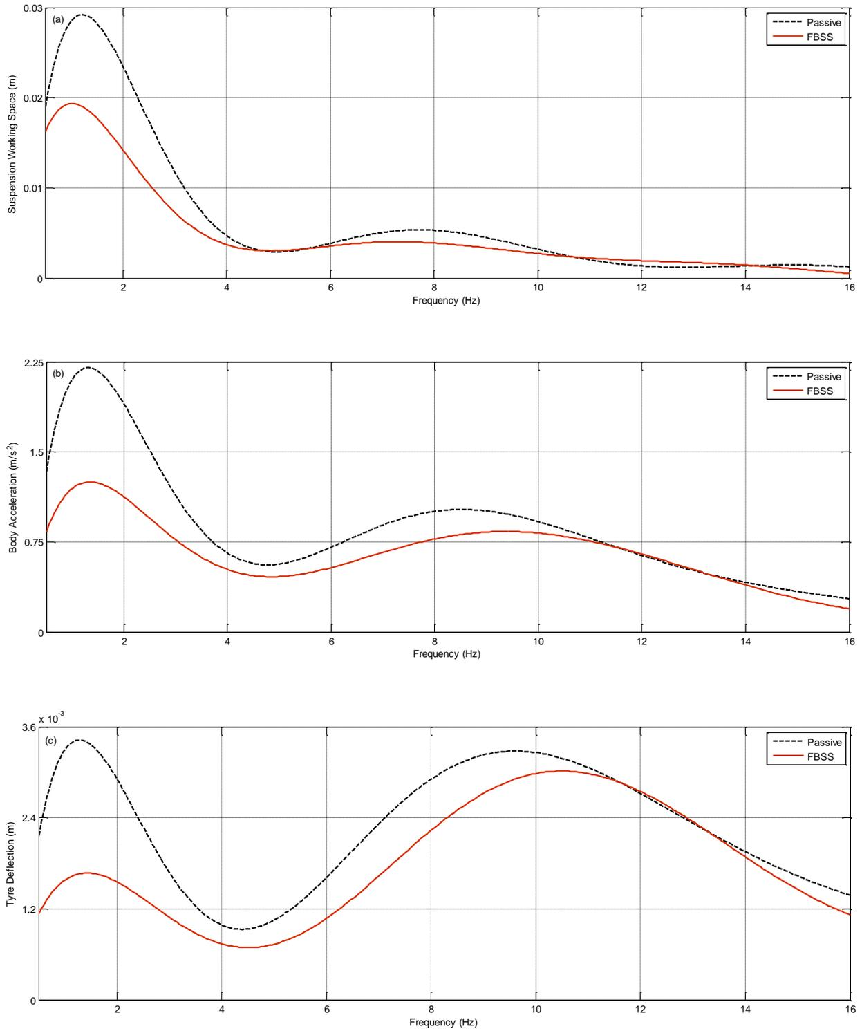
Fig. 8 The FFT of the passive and active vehicle suspension systems.
