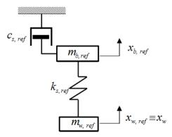
Fig. 3 The reference sky-hook damped model [16]
