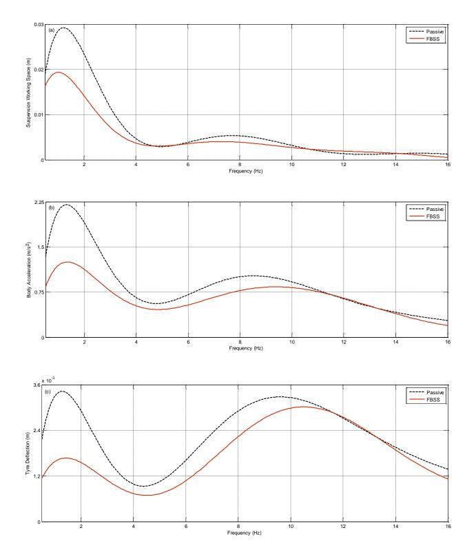
Fig. 8 The FFT of the passive and active vehicle suspension systems. a- SWS b- BA c- DTL
