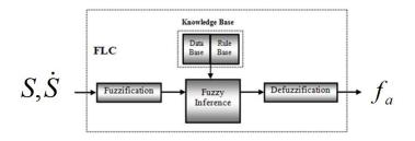
Fig. 4 Fuzzy logic control architecture
