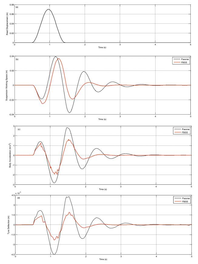
Fig. 7 The passive and active vehicle suspension systems performance under road bump excitation. a- Road Displacement b- SWS c- BA d- DTL
