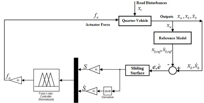
Fig. 2 The proposed FBSS controller for active vehicle suspension
