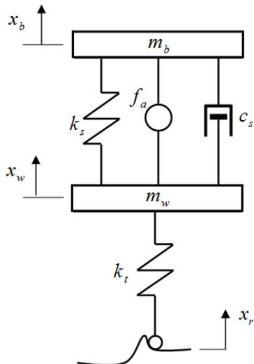
Fig. 1 Quarter vehicle active suspension model.
