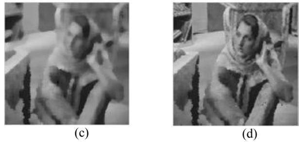
Figure. 8: (a) Original Image, (b) Image contaminated with aleatory noise , (c) Filtered image using static median of size  $11 \times 11$ , (d) Filtered image using proposed fuzzy median filter
