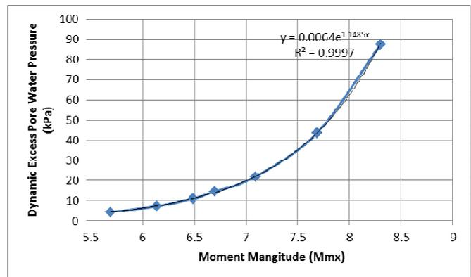
Fig.6 Variation of the dynamic excess pore water pressure with moment mangitude due to horizontal component of earthquake
