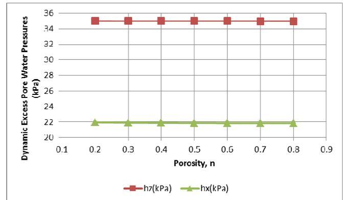
Fig. 2 Variations of the shear wave velocity and the dynamic excess pore water pressures with the porosity.
