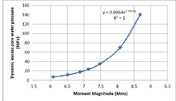
Fig.5 Variation of the dynamic excess pore water pressure with moment mangitude due to vertical component of earthquake
