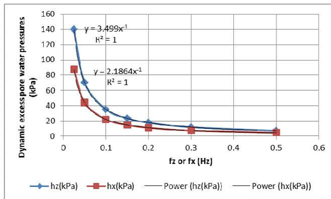
Fig. 4 Variations of the dynamic excess pore water pressures with the frequencies of earthquakes in vertical and horizontal directions.
