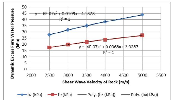
Fig. 9 Variations of the dynamic excess pore water pressures with the shear wave velocity of hard rock.
