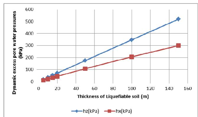
Fig. 3 Variations of the dynamic excess pore water pressures with the thickness of the liquefiable soil (soil No.2).
