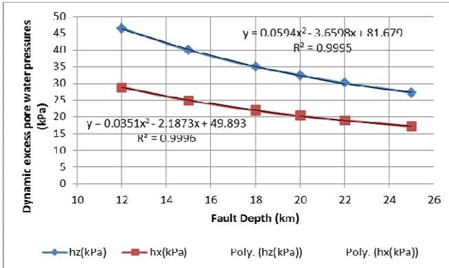
Fig. 7 Variations of the dynamic excess pore water pressures with the fault depth of earthquakes.
