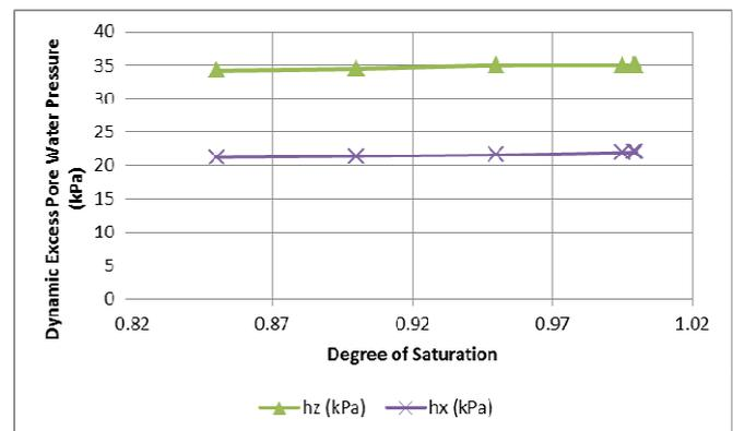
Fig. 1 Variations of the dynamic excess pore water pressures with the degree of saturation
