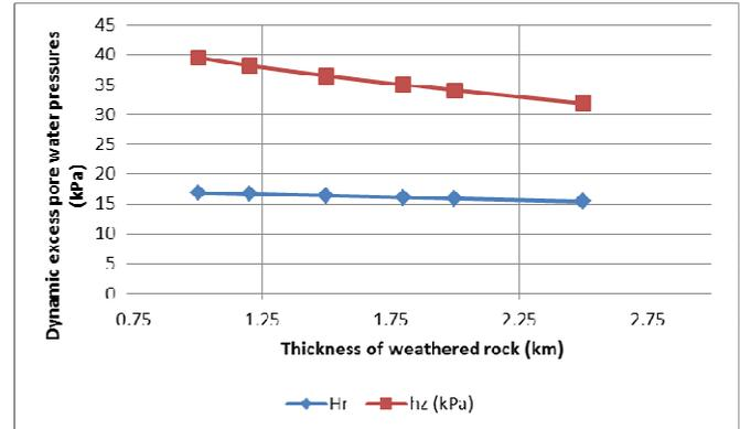
Fig. 8 Variations of the dynamic excess pore water pressures with the thickness of weathered rock.
