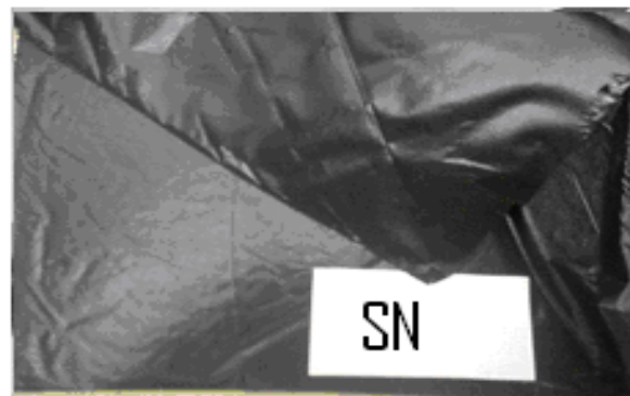
Fig.4 Laying of siloxanic rubber and nanocarbon mixture without plated netting (SN)
