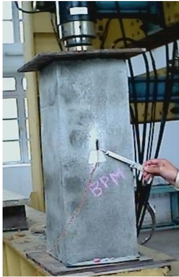
Fig. 2 Plastered specimen with a strain gage at mid-height
