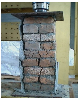
Fig. 7 Specimen near failure
