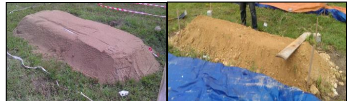
Fig. 1 small model of soil trail embankment built up using sandy soil (left) and lateritic (right) soil
