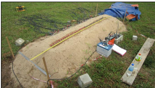
Fig. 2 soil model 1 (sandy soil) tested by 2D electrical resistivity imaging
