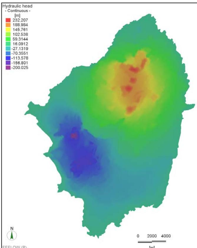
Fig. 9 simulated hydraulic head for October 2010.
