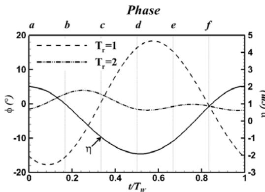
Fig. 4 Roll angle ( $\phi$ ) profiles with wave elevation ( $\eta$ ) during one period normalized by each wave period with phases of vorticity contour in Fig. 5 at the wave periods of  $T_r = 1$  and  $T_r = 2$
