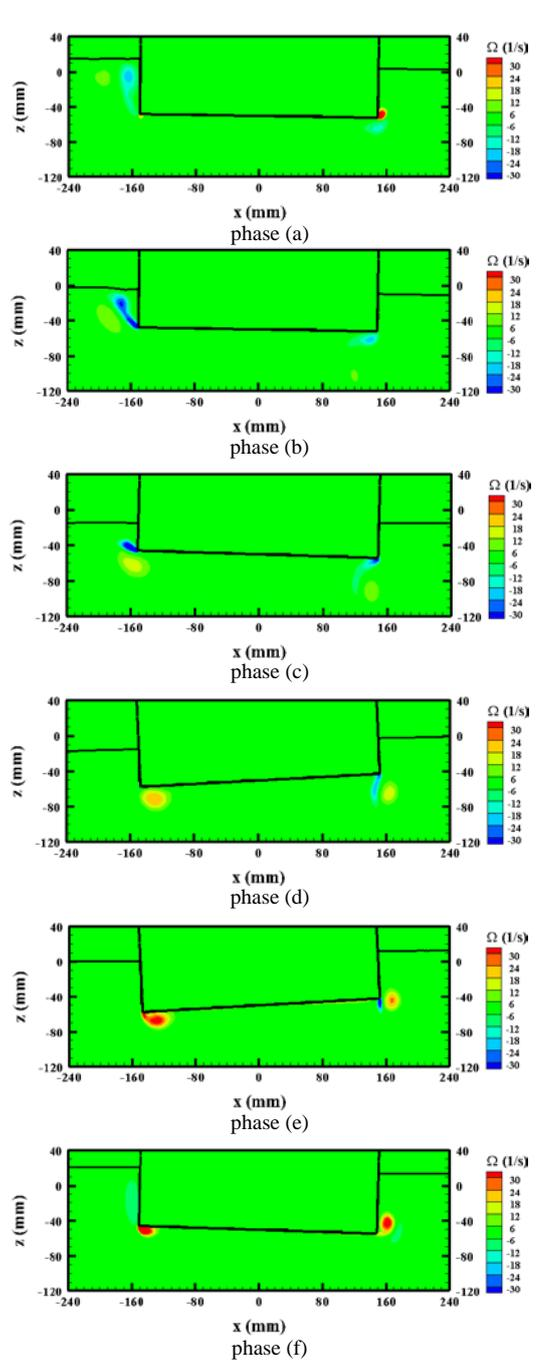
Fig. 5 Vorticity contours of  $T_r = 1$  (left column) and  $T_r = 2$  (right column): phase number of each subtitle matches to the phase in Fig. 4
