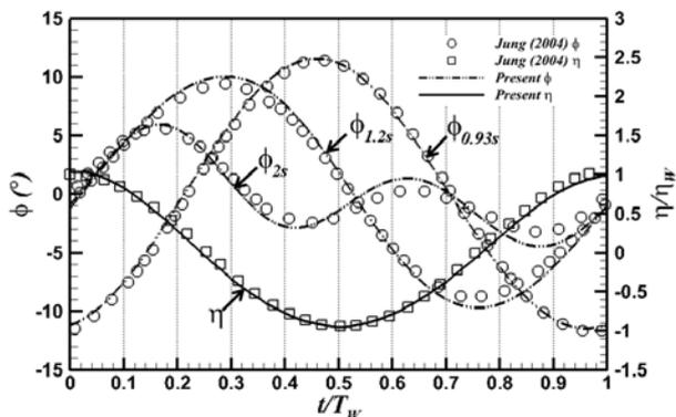
Fig. 3 Wave elevation ( $\eta$ ) and roll angle ( $\phi$ ) profiles during one period normalized by each wave period for  $T_W = 0.93s, 1.2s, 2s$
