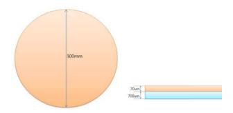
Fig. 14 Wafer model in cases (Aluminum and Silicon)
