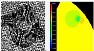
Fig. 10 Contours of static pressure and result of case2 analysis(HYPER-MESH, FLUENT)
