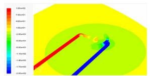
Fig. 3 Contours of static pressure of wafer hole and u line (FLUENT)
