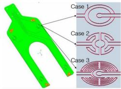
Fig. 4 U Line and hole for the different cases with air bearing principle
