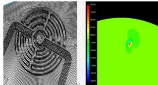
Fig. 11 Contours of static pressure and result of case3 analysis(HYPER-MESH, FLUENT)
