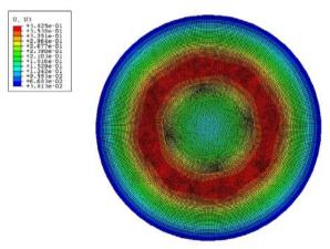
Fig. 12 Wafer analysis by Case wafer displacement(ABAQUS 5.7)
