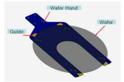
Fig. 2 Wafer hand modeling of upper hand plate, under hand plate and wafer guide(Pro-E)
