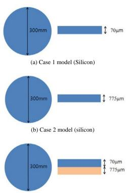
(c) Case 3 model (Aluminium and Silicon) **Fig. 5** Wafer model in each cases
