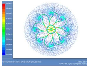
Fig. 13 Wafer chuck analysis with pressure (upper side) and Velocity (under side) with Fluent
