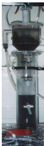
Fig. 1. Laboratory-scale UASB reactor used in this work.
