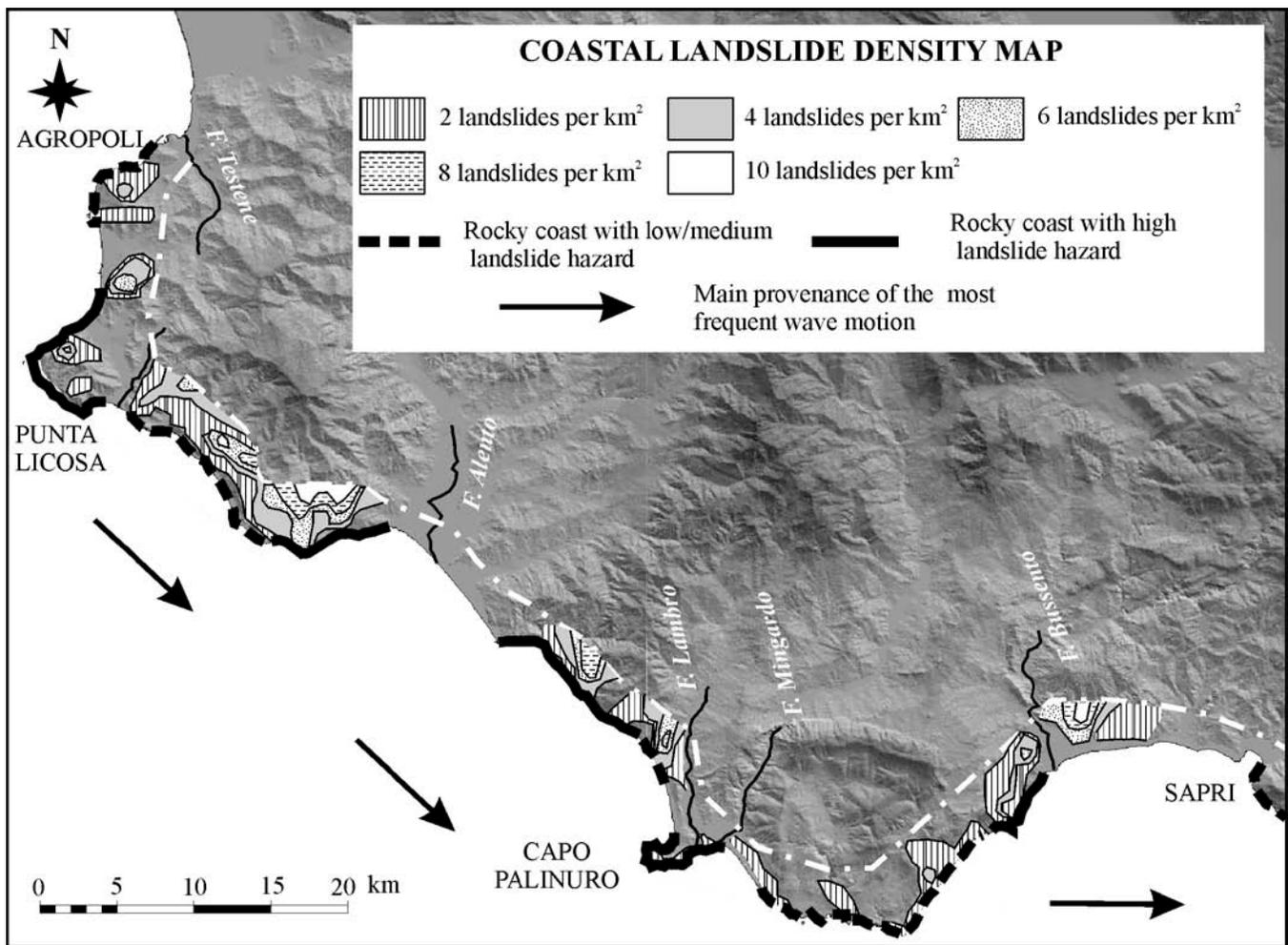
Fig. 7 Landslide density map of the Cilento shoreline
