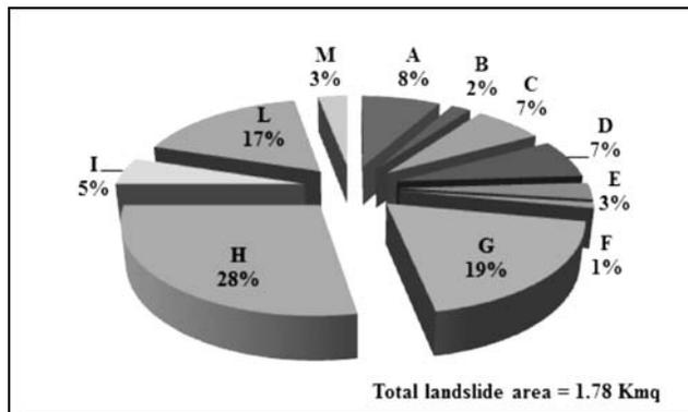
Fig 5 Frequency of typologies and areas of the landslides affecting the studied coast. Key: A = active debris flows; B = inactive slow earth flows; C = active slow earth flows; D = dormant slow earth flows; E = rock-falls; F = active rotational slides; G = suspended rotational slides; H = dormant rotational slides; I = active complex slide-flows; L = dormant complex slide-flows; M = active translational slides
