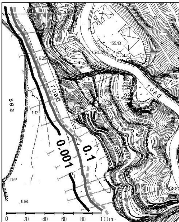
Fig 9 Map of reach boundary probability lines of 0.1 (41.3°), 0.01 (39.5°), and 0.001 (36.9°) for a coastal slope
