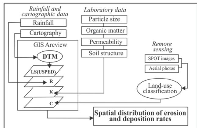
Fig 8 Conceptual flow diagram used in order to apply USPED
