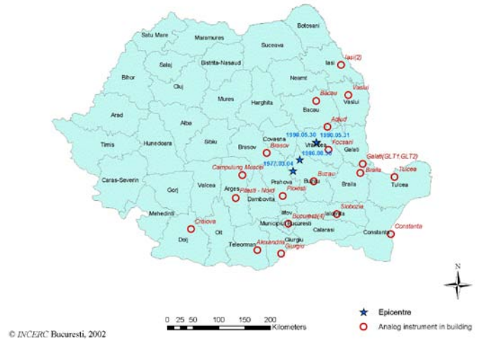
Fig. 4 INCERC seismic stations which provided records in seismic instrumented buildings during Vrancea earthquakes of 1977, 1986 and 1990 [4]
