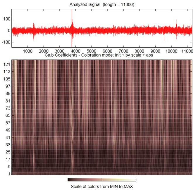
Fig.4 The 2012/11/23 02:08 UMT seismic event, recorded at 3rd floor of new building (3NB) accelerometer, North-South component (NS) 9F8E accelerometer , analyzed with Wavelet Transform , WV family db (level 2)
