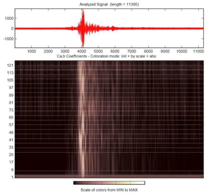
Fig.10 2013/01/05 02:04 UMT seismic event, recorded at 3rd floor old building (3OB) accelerometer, North-South component (NS) A392 accelerometer , analyzed with Wavelet Transform , WV family db (level 2)
