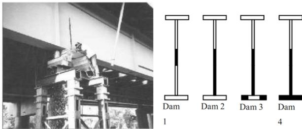
Fig.1 *Damage Detection Study of the I-40 Bridge over the Rio Grande in New Mexico, USA. Left figure: electric saw cutting cause damage in the bridge girder right figure: The levels of introduced damage in the girder (the shaded area is the reduced cross-section)[7].*
