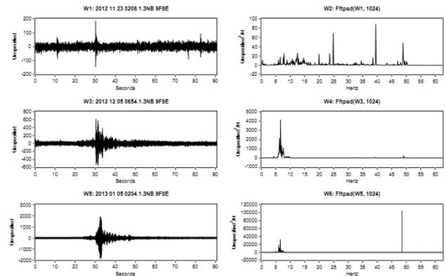
Fig.7 FFT based PSDs for the previous events (Figs 3,4 &5)
