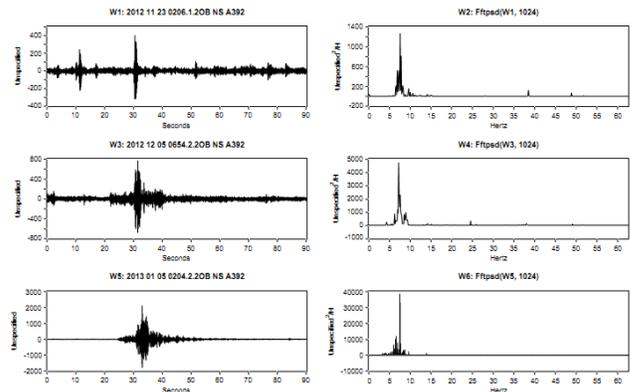
Fig.11 FFT based PSD for the previous events (Figs 7,8 &9)
