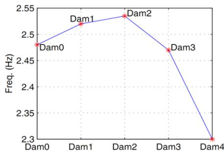
Fig.2 *The change of fundamental frequency on I-40 Bridge related to the damage levels presented in Figure 2.4[7]*
