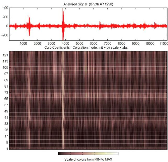
Fig.8 2012/11/23 02:08 UMT seismic event, recorded at 3rd floor old building (3OB) accelerometer, North-South component (NS) A392 accelerometer , analyzed with Wavelet Transform , WV family db (level 2)
