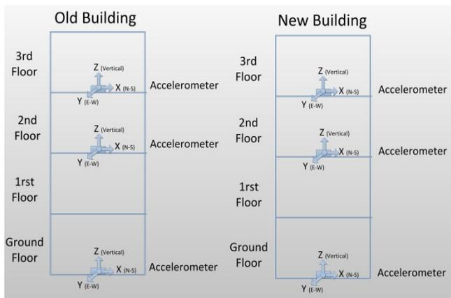
Fig.2 Schematic Deployment of the accelerometers in the buildings
