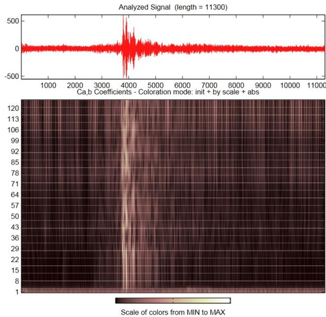
Fig.5 2012/12/05 06:54 UMT seismic event, recorded at 3rd floor new building (3NB) accelerometer, North-South component (NS) 9F8E accelerometer , analyzed with Wavelet Transform , WV family db (level 2)
