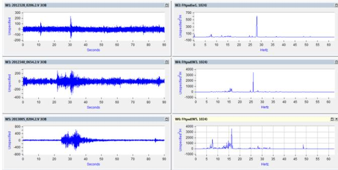
Fig.12 FFT based PSDs for the previous events (up 2012/11/23 02:08 UMT, middle 2012/12/05 06:54 UMT and lower 2013/01/05 02:04 UMT) for the old building (Vertical component)
