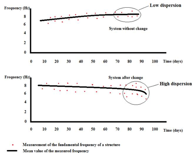
Fig.1 Low and high dispersion of fundamental frequency of a structure
