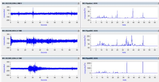
Fig.13 FFT based PSDs for the previous events (up 2012/11/23 02:08 UMT, middle 2012/12/05 06:54 UMT and lower 2013/01/05 02:04 UMT) for the new building (Vertical component)
