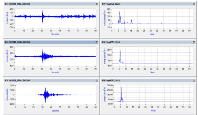
Fig.14 FFT based PSDs for the previous events (up 2012/11/23 02:08 UMT, middle 2012/12/05 06:54 UMT and lower 2013/01/05 02:04 UMT) for the old building (East-West component)
