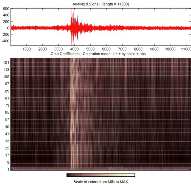
Fig.9 2012/12/05 06:54 UMT seismic event, recorded at 3rd floor old building (3OB) accelerometer, North-South component (NS) A392 accelerometer , analyzed with Wavelet Transform , WV family db (level 2)
