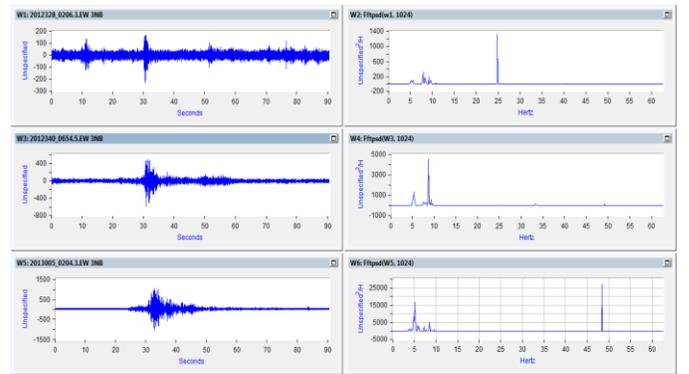
Fig.15 FFT based PSDs for the previous events (up 2012/11/23 02:08 UMT, middle 2012/12/05 06:54 UMT and lower 2013/01/05 02:04 UMT) for the new building (East-West component)
