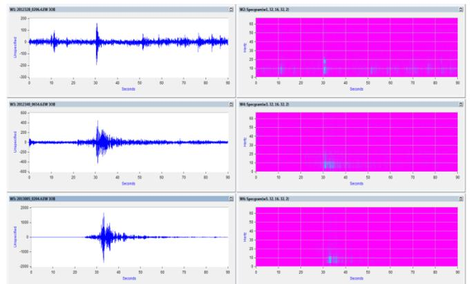
Fig.16 Spectrogram for the previous events (up 2012/11/23 02:08 UMT, middle 2012/12/05 06:54 UMT and lower 2013/01/05 02:04 UMT) for the old building (East-West component)
