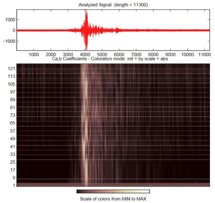
Fig.6 2013/01/05 02:04 UMT seismic event, recorded at 3rd floor new building (3NB) accelerometer, North-South component (NS) 9F8E accelerometer , analyzed with Wavelet Transform , WV family db (level 2)
