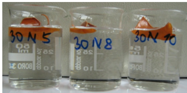
Fig. 2 Tested samples with 30 % of crotonaldehyde at the beginning of dissolving in distilled water. Time of cross-linking: 5 minutes (left sample), 8 minutes (middle sample), 10 minutes (right sample).
