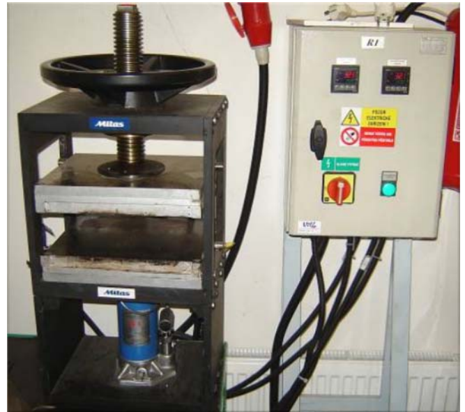
Fig. 9 Laboratory press for manufacturing of thermo-insulating panel samples
