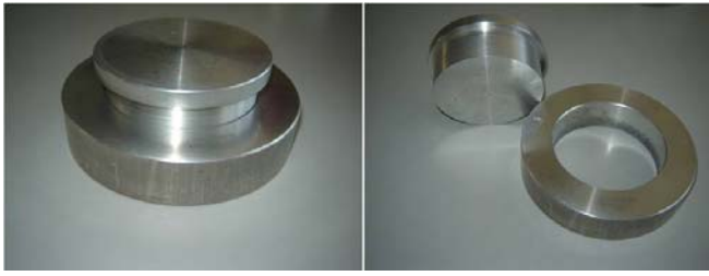
Fig.8 Form for manufacturing of thermo-insulating panel samples
