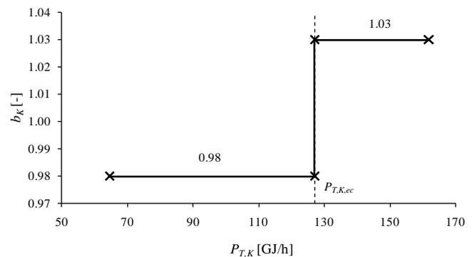
Fig. 10 Increment of heat consumption of boilers K23 and K24
