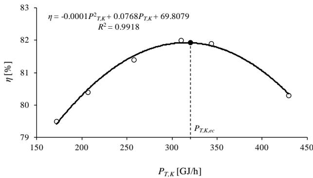
Fig. 5 Efficiency curve of boilers K27, K28 and K29
