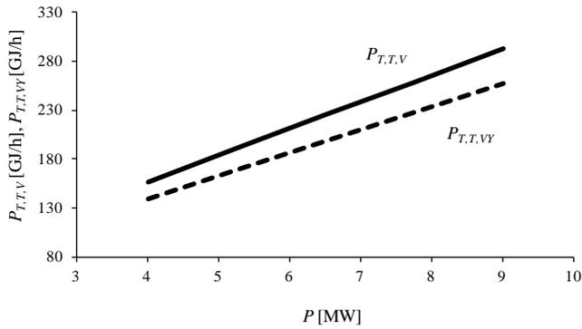
Fig. 16 Back-pressure turbine TG26 characteristics
