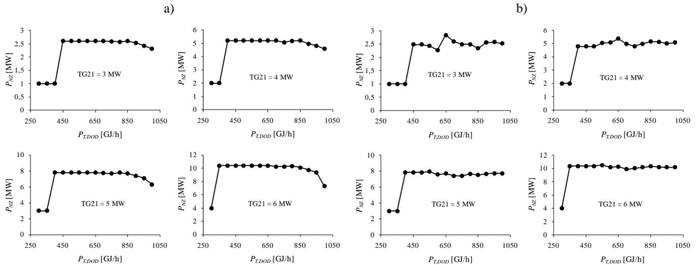
Fig. 23 Output courses of functional dependence  $P_{NZ} = f(P_{T,DOD})$ , for separate constant values of electric output on TG21, which was obtained by using simplex method (a) and genetic algorithm (b)
