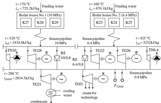
Fig. 2 Scheme of combined production of heat and electric energy
