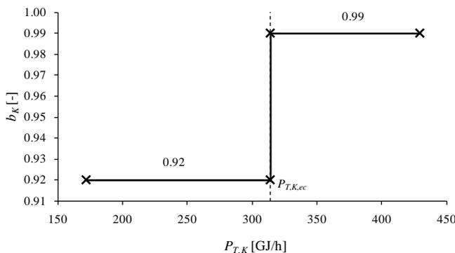
Fig. 7 Increment of heat consumption of boilers K27, K28 and K29
