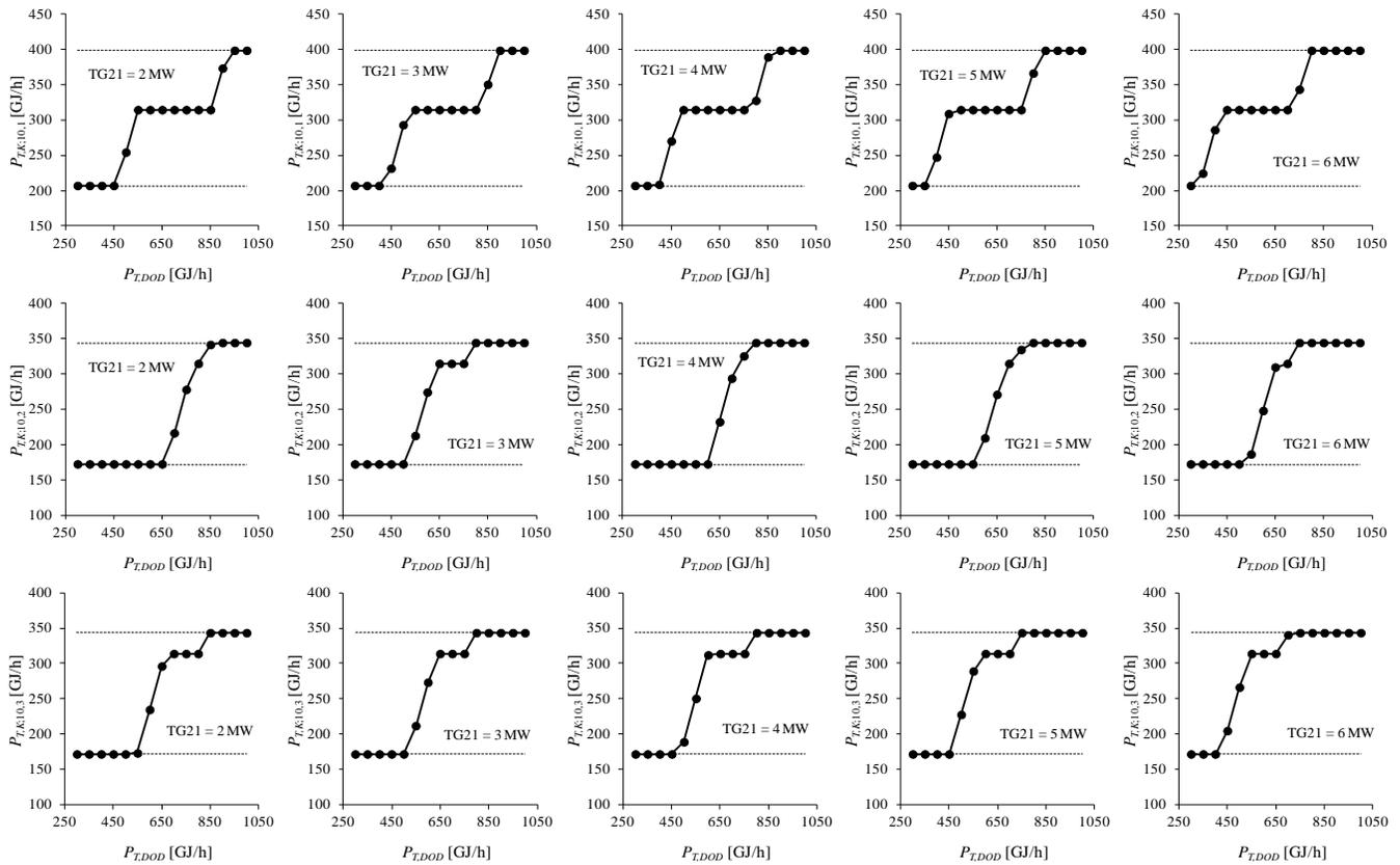
Fig. 20 Output courses of functional dependence  $P_{T,K} = f(P_{T,DOD})$ , for separate constant values of electric output on TG21 and for boilers K27, K28, K29, which were obtained by using simplex method
