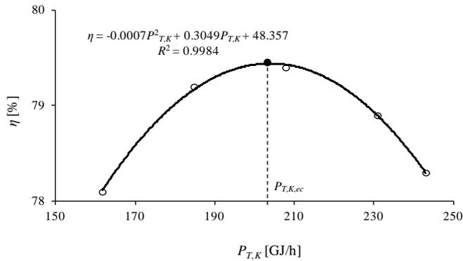
Fig. 11 Efficiency curve of boiler K25
