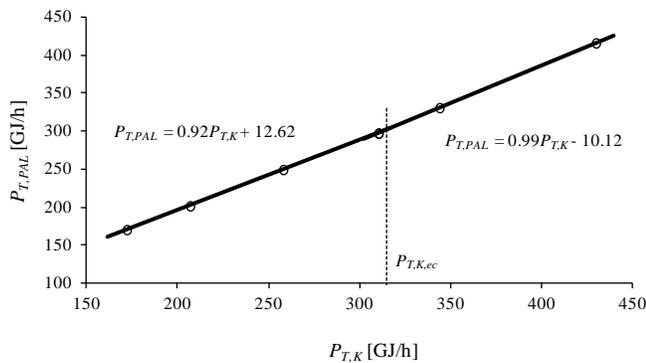
Fig. 6 Linear replacement of consumption characteristic of boilers K27, K28 and K29
