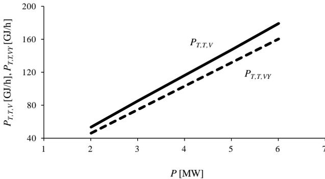
Fig. 18 Condensing turbine TG21 characteristics
