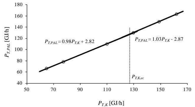
Fig. 9 Linear replacement of consumption characteristic of boilers K23 and K24
