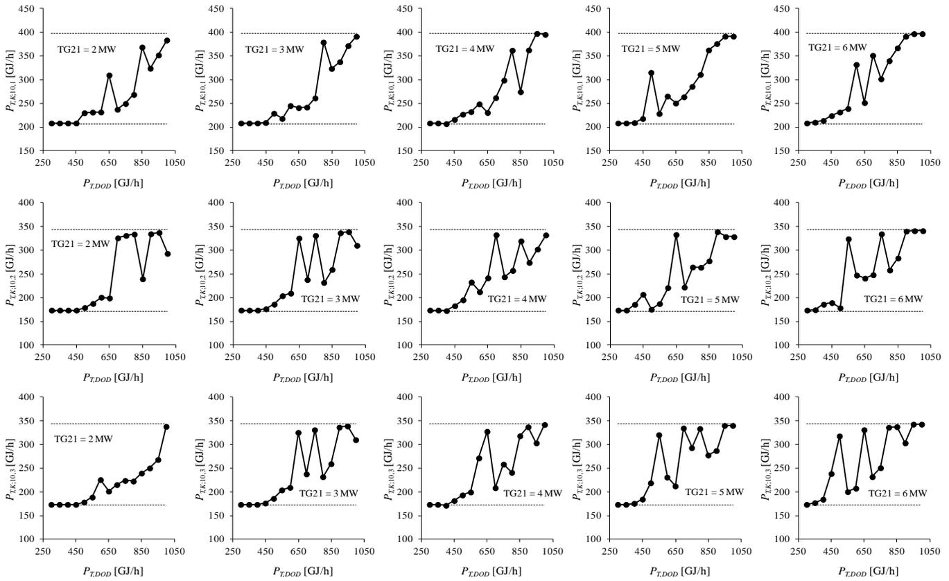
Fig. 22 Output courses of functional dependence  $P_{T,K} = f(P_{T,DOD})$ , for separate constant values of electric output on TG21 and for boilers K27, K28, K29, which were obtained by using genetic algorithm
