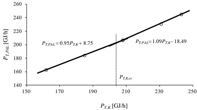
Fig. 12 Linear replacement of consumption characteristic of boiler K25
