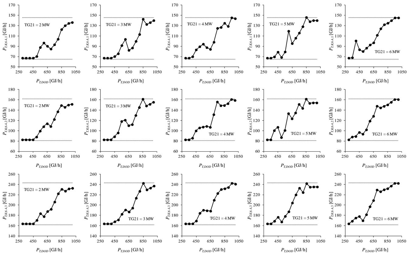
Fig. 21 Output courses of functional dependence  $P_{T,K} = f(P_{T,DOD})$ , for separate constant values of electric output on TG21 and for boilers K23, K24, K25, which were obtained by using genetic algorithm
