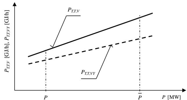
Fig. 4 Consumption characteristic of turbine
