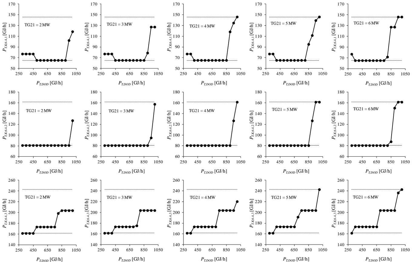
Fig. 19 Output courses of functional dependence  $P_{T,K} = f(P_{T,DOD})$ , for separate constant values of electric output on TG21 and for boilers K23, K24, K25, which were obtained by using simplex method
