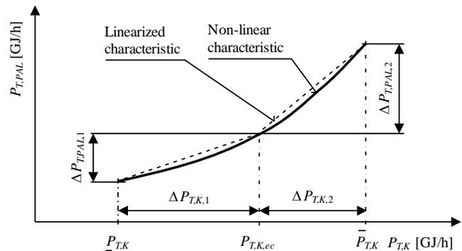
Fig. 3 Consumption characteristic of boiler and its linearization
