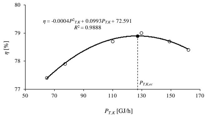
Fig. 8 Efficiency curve of boilers K23 and K24
