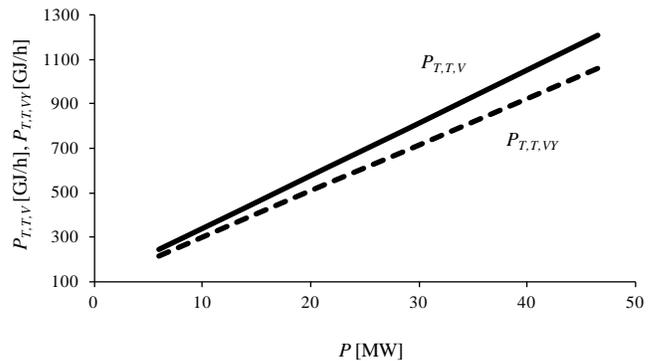
Fig. 14 Back-pressure turbine TG28 characteristics
