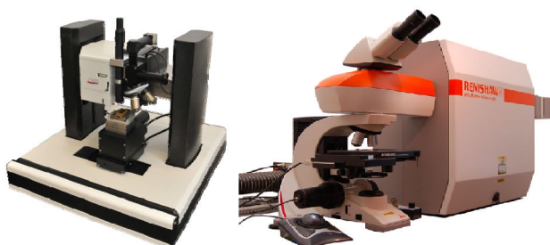
Fig. 5 Instruments used for instrumented microhardness tests (left) and acquiring Raman spectra (right).
