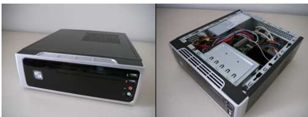
Fig. 2 Suitable HW platform containing x86 Intel Atom 1.6GHz, RAM 1GB/677MHz and 16GB SSD.
