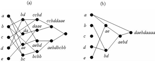
Fig. 8 the structure of network corresponding to (a) point C on Figure 5, (b) point I on Figure 7, in which a, b, c, d and e stand for  $\log \sigma_{\max}$ ,  $\sigma_{\max} / \sigma_u$ ,  $W$ ,  $R$ ,  $\theta$ , respectively.
