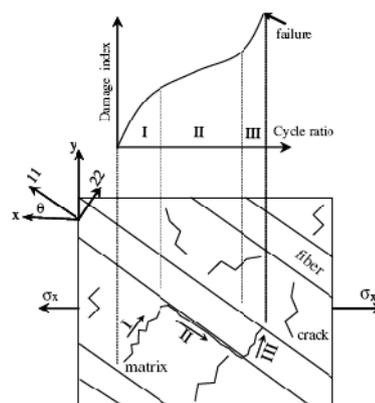
Fig. 1 three regions of cracking mechanism in unidirectional composites
