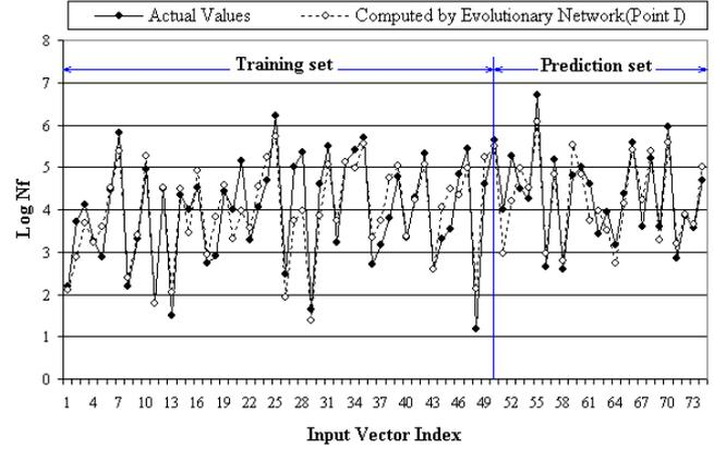
Fig. 10 comparison of actual values with the evolved GMDH model corresponding to optimum point I.
