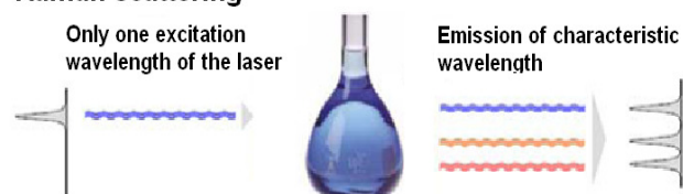
Fig. 1 Differences of light-matter interaction of infrared and Raman spectroscopy
