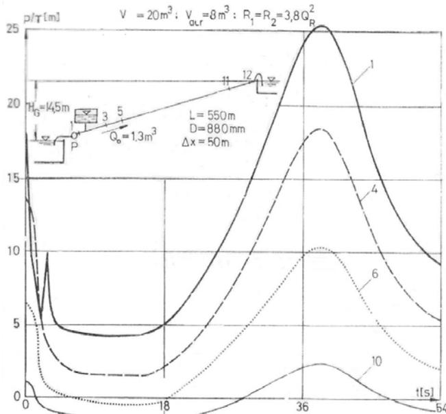
Fig. 10 Old pumping station SRP 4 Seimeni. Pressure values in the discharge duct [11]
