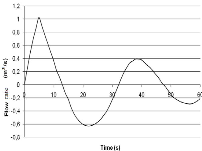
Fig.17 Flow rate for the water change between air chamber and duct
