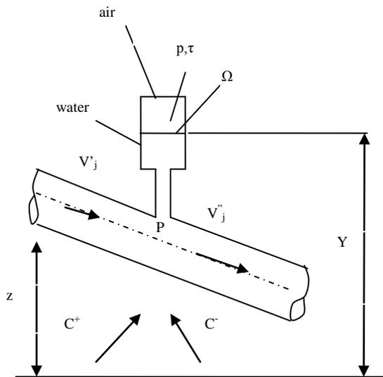
Fig. 2 Calculus node with air chamber
