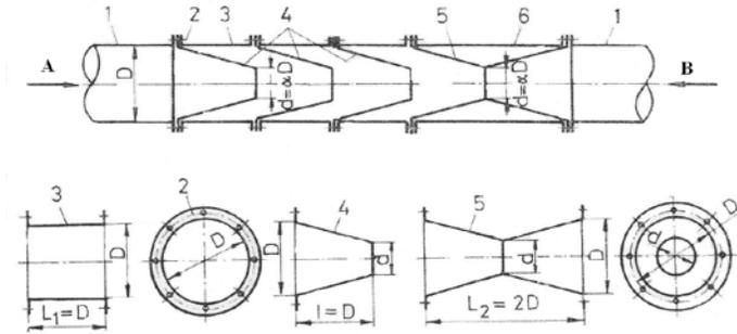
Fig.12 The device with asymmetrical hydraulic resistance, type I.C.H: 1,3-duct; 2- flange; 4- conical nozzle; 5- bi-conical nozzle; 6-duct, [13].
