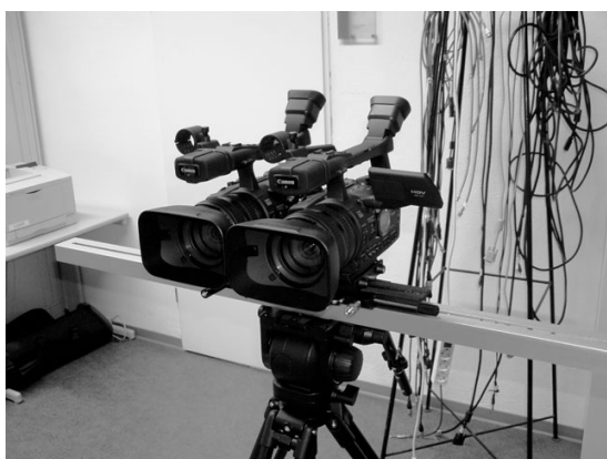
Fig. 14: Stereoscopic camera with adjustable distance between objectives [13]
